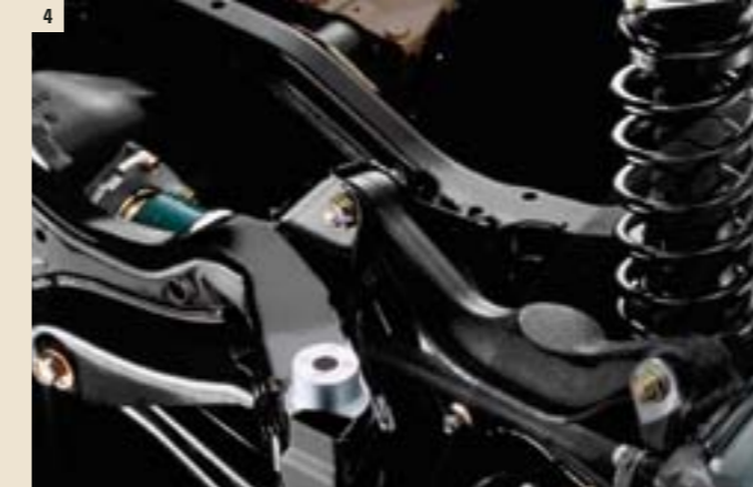
4 A sophisticated, reengineered multi-link rear suspension features newly revised geometry. It's designed to offer greater resistance to roll when cornering, and helps resist squatting during hard acceleration.
