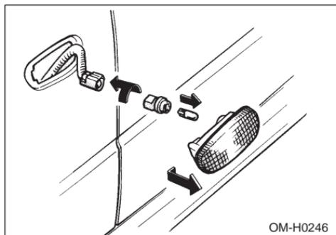
1. Pull the left side of the turn signal light assembly while moving it forward in relation to the vehicle.
