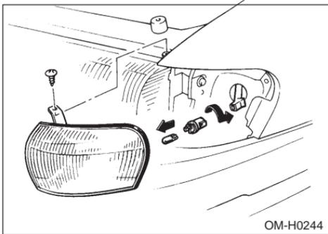
1. Remove the parking light assembly mounting screw located at the top of the headlight assembly using the phillips screwdriver.
