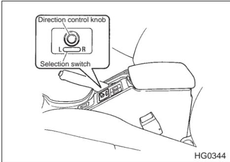
1. Press either end of the selection switch; “L” for the left and “R” for the right.
