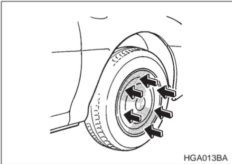
Align the valve with the valve hole in the cover, then fit the cover on the wheel by tapping your hand evenly around the circumference of the cover.
