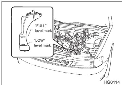
1. Check the coolant level on the outside of the reservoir while the engine is cool.
