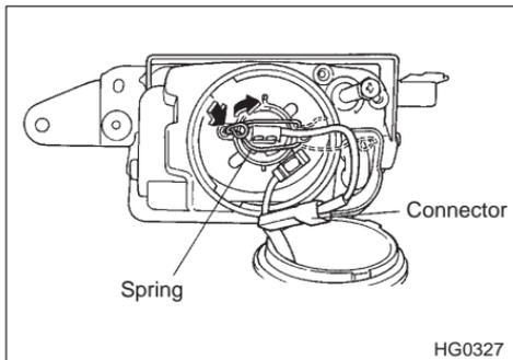
5. Disconnect the connector behind the case cap.
