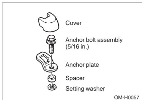
1. Take the anchor kit out and make sure that it is assembled as shown in the illustration above.
