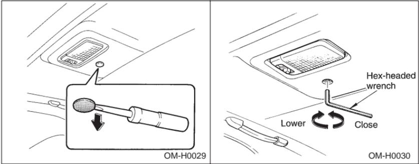
If the sunroof can not be closed with the sunroof switch, you can close the roof manually.
