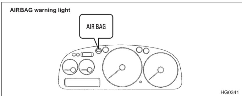
A diagnostic system continually monitors the readiness of the SRS AIRBAG while the vehicle is being driven. The SRS AIRBAG warning light will show normal system operation by lighting for about 6 seconds when the ignition key is turned to the “ON” position.
