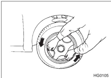
Grasp the wheel cover with both hands by the spokes and twist sharply in a **counterclockwise** direction until you feel the detent release. Now the wheel cover is free from the retention ring.
