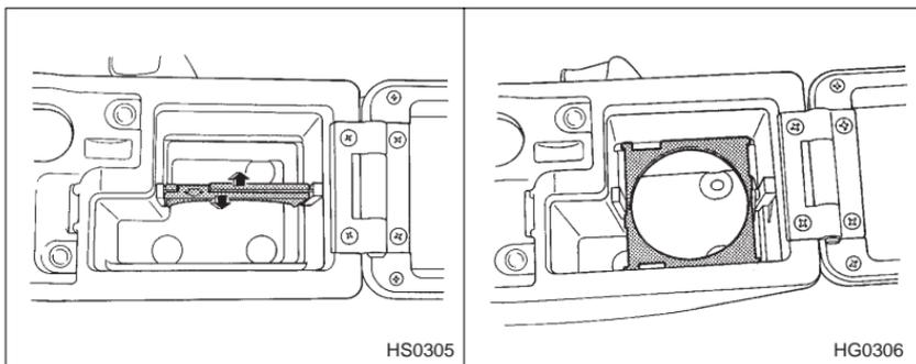
The front passenger's cup holder is built in the center console. To use the cup holder, open the lid of the console and open the holder. When not in use, fold the holder and close the lid.
