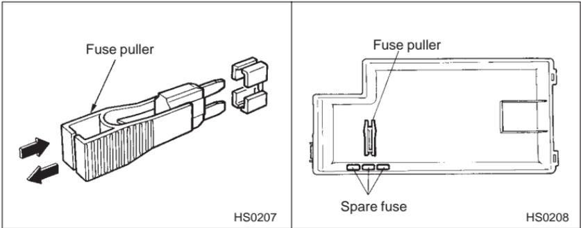
5. Pull out the fuse with the fuse puller provided in the main fuse box cover.
