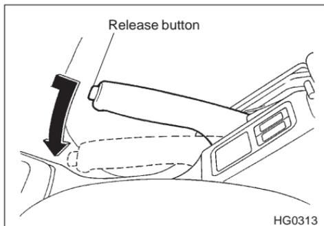
To release the parking brake, pull the lever up slightly, press the release button, then lower the lever while keeping the button pressed.
