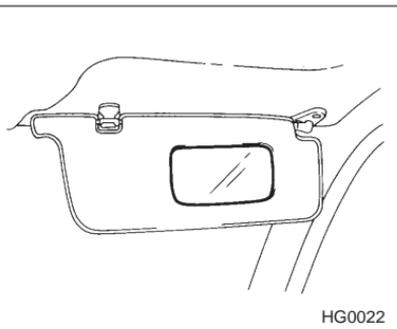
To block out glare, swing down the visors. To use the sun visor at a side window, swing it down and move it sideways.
