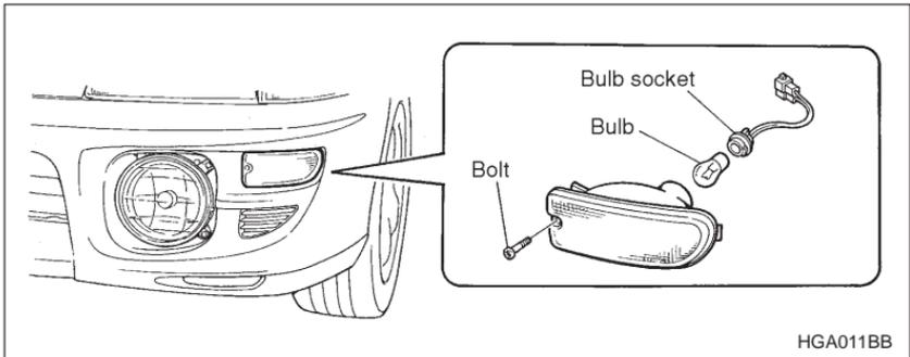
1. Remove the bolt securing the front turn signal light assembly.
