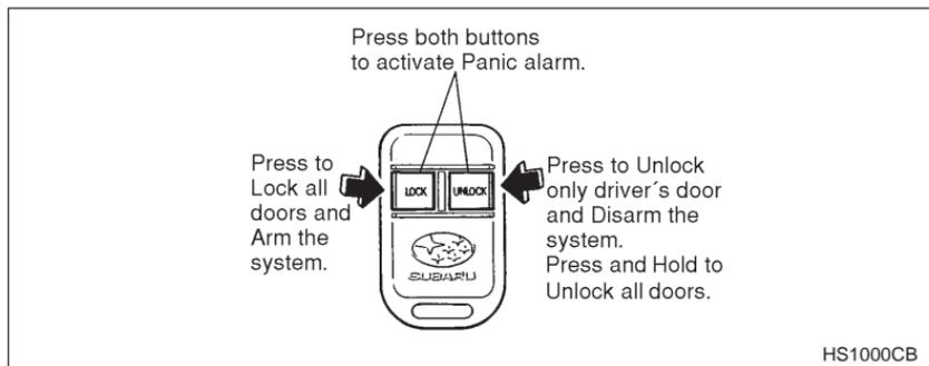
The security system can be programmed to operate with one to four remote transmitters. Each transmitter is powered by an internal 12-volt alkaline battery.
