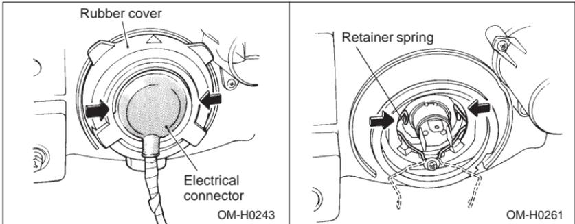
1. Disconnect the electrical connector, then remove the rubber cover.
