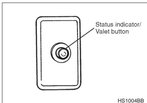
The Status Indicator is a high intensity warning light, located on the dash to the left of the steering wheel. The Status Indicator displays a visual indication of the security system's status while creating a powerful theft deterrent.
