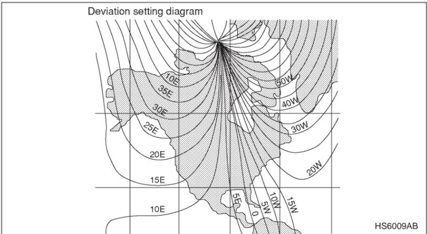
Depending on your location, the following adjustment is required due to the difference between magnetic and geographic North. Refer to the map shown above for the setting most appropriate for your location.
