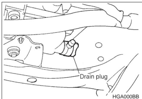
2. Loosen the radiator cap to drain the coolant from the radiator. Then drain the coolant from the reserve tank. Tighten the drain plug securely.
