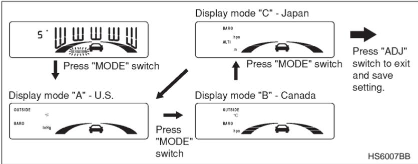
3. Change the measurement units by pressing the "MODE" switch until the proper mode appears.
