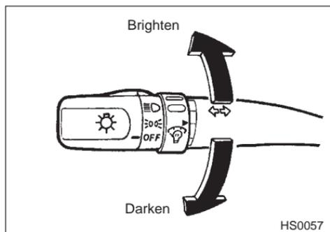
When the lighting switch is in the “ $\text{☀}$ ” or “ $\text{☾}$ ” position, you can adjust brightness of the instrument panel illumination for better visibility.
