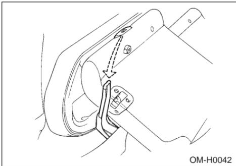
To return the rear seat to its original position, raise the seatback and seat cushion until it locks into place and make sure that they are securely locked.
