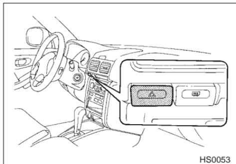
Day or night, if your vehicle becomes a traffic hazard, use the hazard warning flasher. Avoid stopping on the road. It is best to safely pull off the road if a problem occurs. The hazard warning flasher can be activated regardless of the ignition switch position.
