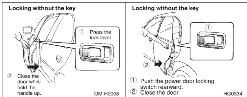
To lock the **front door** from the outside without the key, press the end of the lock lever down on the door and hold the outside door handle up while closing the door.
