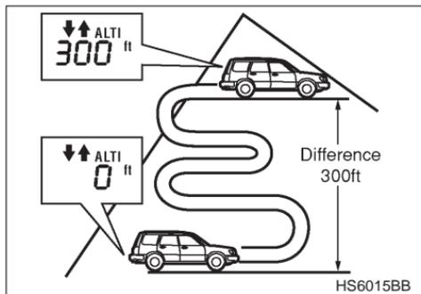
The altimeter indicates the relative elevation.
