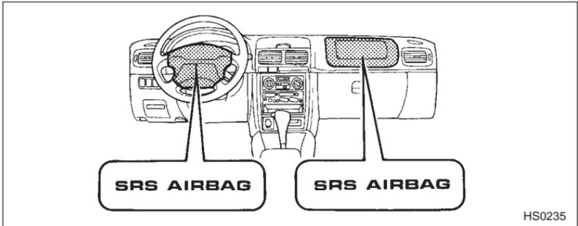
The driver's side SRS AIRBAG is stored in the center portion of the steering wheel. The passenger's side SRS AIRBAG is stored near the top of the dashboard under the cover marked "SRS AIRBAG".
