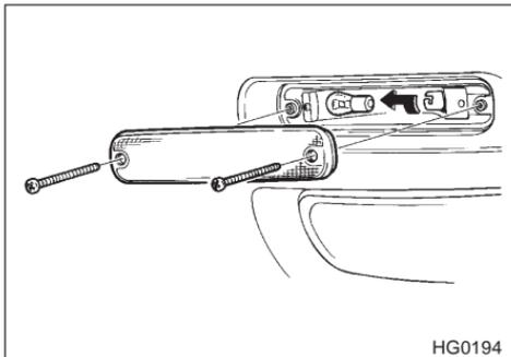
1. Remove the front turn signal light assembly mounting screws using the phillips screwdriver.
