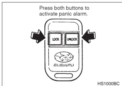
Pressing both buttons together on the remote transmitter activates the Panic feature, sounding the siren and flashing the parking lights. Panic is designed to bring attention to the vehicle and surrounding area. Press either button on the transmitter to turn off the Panic alarm.
