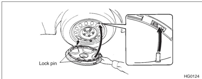
2. Grasp the wheel cover with both hands by the spokes and twist sharply in a **clockwise** direction until you feel the detent locking. After twisting the wheel cover, make sure the wheel cover is locked securely by lightly turning the wheel cover right and left.
