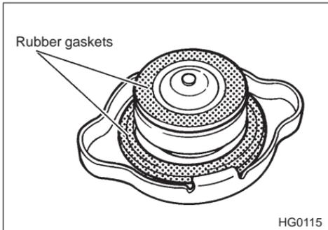
4. Put the radiator cap back on and tighten firmly. At this time, make sure that the rubber gaskets in the radiator cap is correctly in place.
