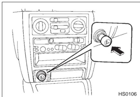
The cigarette lighter operates only when the ignition switch is in the “ON” and “ACC” position.
