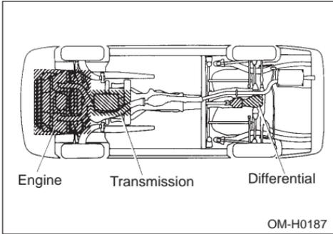
Inspect the following for oil leaks:
