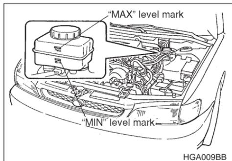
Check the fluid level on the outside of the reservoir. If the level is below “MIN”, add the recommended brake fluid to “MAX”.
