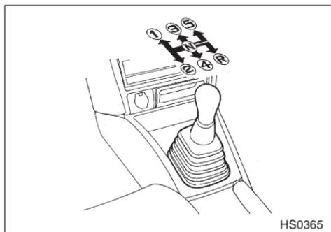
The shift pattern is shown on the shift lever knob. When shifting from 5th gear to reverse gear, first return the shift lever to neutral position then
