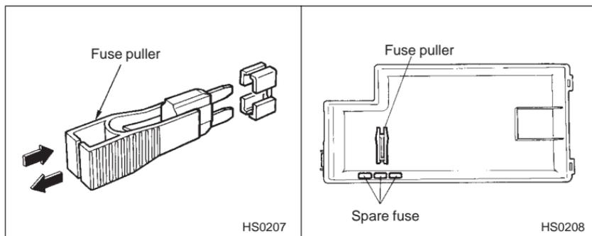
4. Pull out the fuse with the fuse puller. The fuse puller is stored in the main fuse box cover in the engine compartment.
