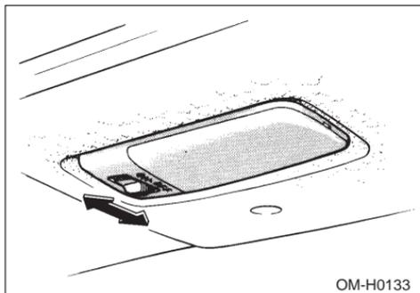
The interior light switch has three positions:
