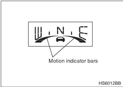
1. 1.8 mile/h (2.8 km/h) of vehicle speed ... 1 second interval bar motion.
