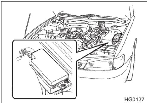
The main fuses and fusible link are designed to melt during an overload to prevent damage to the wiring harness and electrical equipment. Check the main fuses and fusible link if any electrical component fails to
