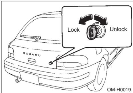
To unlock the rear gate, insert the key in the keyhole and turn it clockwise. To lock the rear gate, insert the key in the keyhole and turn it counterclockwise. If your vehicle is equipped with power door locks, the rear gate can also be locked and unlocked through use of the power door lock system. Refer to the Power Door Locks section in this chapter.
