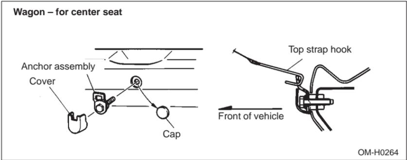
2. Remove the cover of the anchor installation point.
