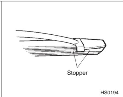
6. Install the wiper blade assembly to the wiper arm. Make sure that it locks in place.
