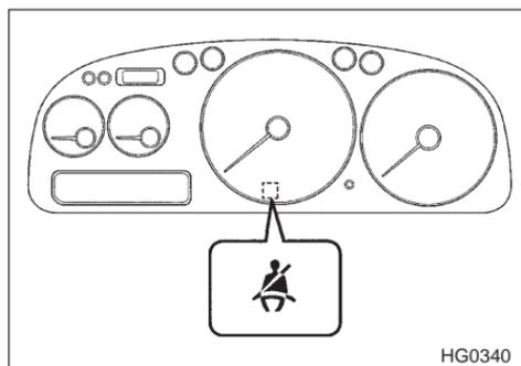
Your vehicle is equipped with a seat belt warning device at the driver's seat.
