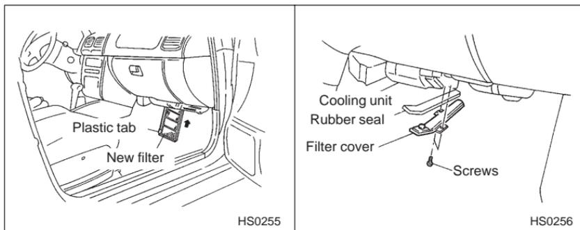
3. Insert a new filter with the plastic tab facing forward.
