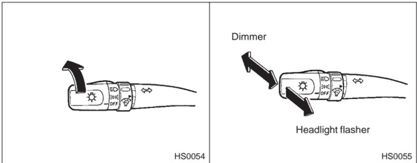
The light switch operates only when the ignition switch is in the “ON” position.
