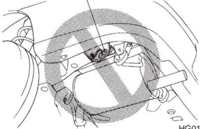
The towing eyelets should be used only in an emergency (e.g., to free a stuck vehicle from mud, sand or snow).
