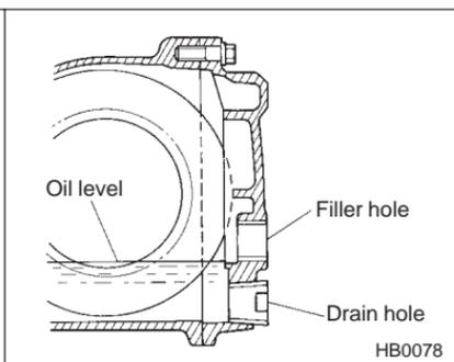
Remove the plug from the filler hole and check the oil level. The oil level should be kept even with the bottom of the filler hole. If the oil level is below the bottom edge of the hole, add oil through the filler hole to raise the level.
