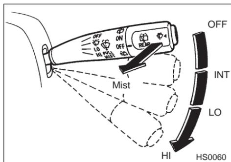
To turn the wipers on, push the wiper control lever down.
