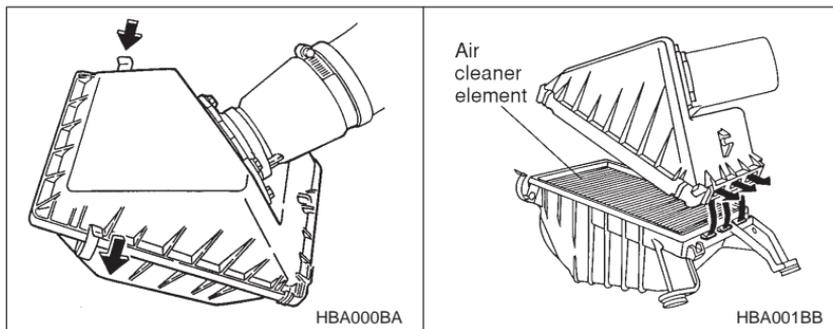
1. Unsnap the two clamps holding the air cleaner case cover.
