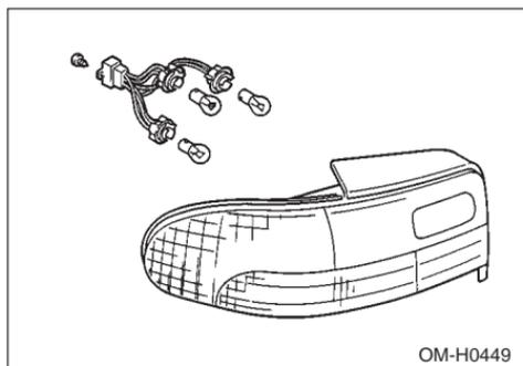
2. Remove the bulb holder from the rear combination light assembly by turning it counterclockwise.
