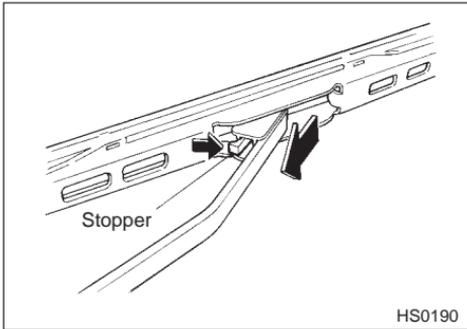
3. Grasp the locked end of the blade rubber assembly and pull it firmly until the stoppers on the rubber are free of the metal support.
