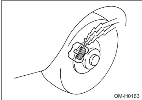
The front disc brake has an audible wear indicator on the brake pads. For RS models, the right side rear disc brake also has a audible wear indicator. If the brake pads wear close to their service limit, the wear indicator makes a very audible scraping noise when the brake pedal is applied.
