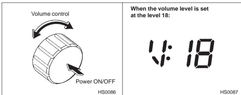
The same knob is used for both power (on/off) and volume control. The radio is turned on and off by pushing the knob and the volume is controlled by turning the knob.
