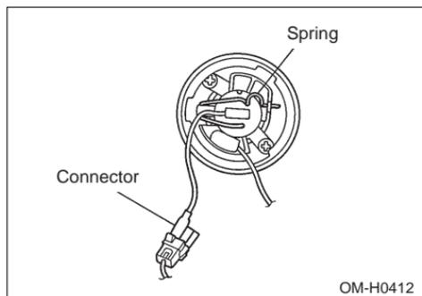
4. Disconnect the connector behind the case cap.
