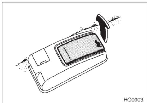
Pull the trunk lid release lever upward.
