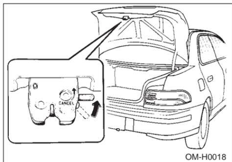
The inside trunk lid release can be cancelled to help prevent unauthorized entry into the trunk. To cancel the trunk lid release, set the lid release cancel lever (located on the inside of the trunk lid, mounted to the trunk lid latch) to the "CANCEL" position. When this lock is in the "CANCEL" position, the trunk can be opened only by the master key.
