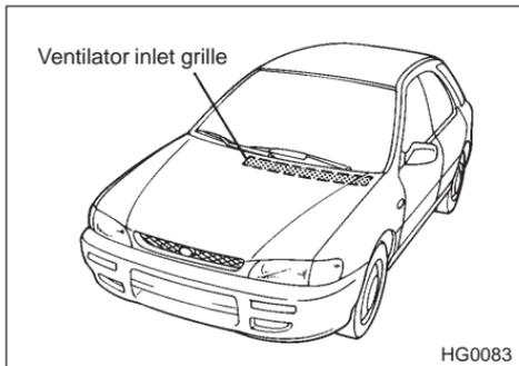
Always keep the front ventilator inlet grille free of snow, leaves, or other obstructions to ensure efficient heating and defrosting. Since the condenser is located in front of the radiator, this area should be kept clean
