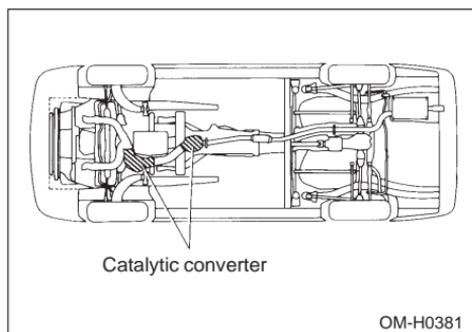
The catalytic converter is installed in the exhaust system. It serves as a catalyst to reduce HC, CO and NO<sub>x</sub> in exhaust gases, thus providing cleaner exhaust.
