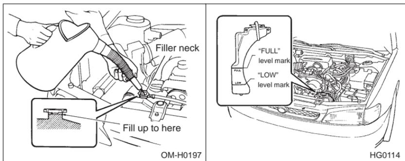
3. Slowly pour the coolant and fill to the radiator filler neck and to the reserve tank's "FULL" level mark. Do not pour the coolant too quickly, as this may lead to insufficient air bleeding and trapped air in the system.
