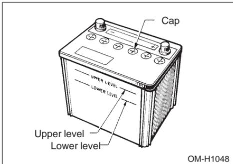
It is unnecessary to periodically check the battery fluid level or periodically refill with distilled water.
