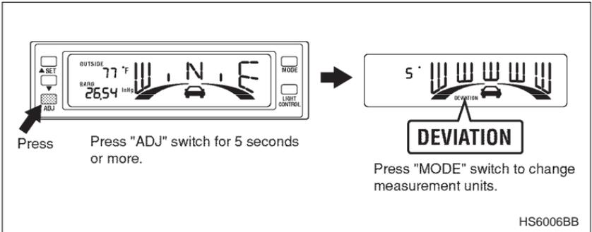
1. Turn on the ignition switch to the “ACC” position and the display shows the default English measurement units.
