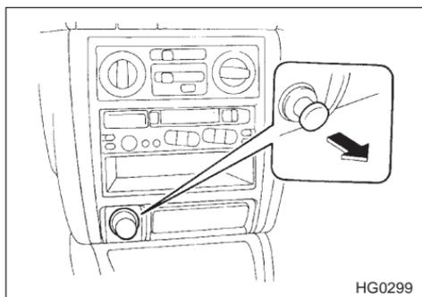
The electrical power socket located on the lower part of the instrument panel can be used as cigarette lighter socket. A cigarette lighter plug is an optional accessory. It is available from your SUBARU dealer. If smoking is not desired, always put the cap on the socket to prevent any foreign object from entering it.
