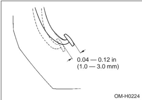
Stop the engine and firmly depress the brake pedal several times. Lightly press the brake pedal down by finger to check the free play with a force of less than 10 N (2 lb., 1 kg).
