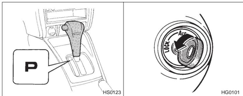
The key can be turned from “ACC” to “LOCK” only when the selector lever is in the “P” position.
