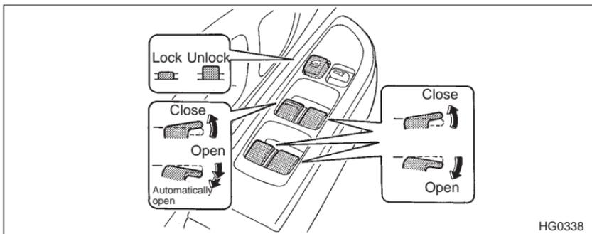
All door windows can be controlled by the power window switch cluster at the driver side door.
