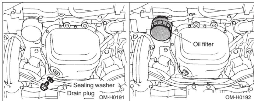
6. Remove the oil filter with an oil filter wrench.
