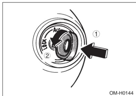
The key can be turned from “ACC” to “LOCK” only when the key is pushed in while turning it.
