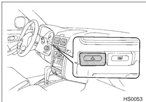
The hazard warning flasher is used to warn other drivers when you have to park your vehicle under emergency conditions. The hazard warning
