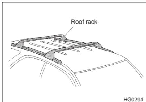
When you carry cargo on the roof using the roof rack, never exceed the maximum load limit explained below. In addition, be careful that your vehicle does not exceed the Gross Vehicle Weight Rating (GVWR) and front and rear Gross Axle Weight Rating (GAWR). See the Loading Your Vehicle section in chapter 7 for information on loading cargo into or onto your vehicle.
