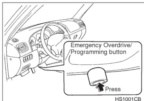
If your remote transmitter fails to operate, the system can be disarmed using the Emergency Override/Programming button. Follow the procedure below:
