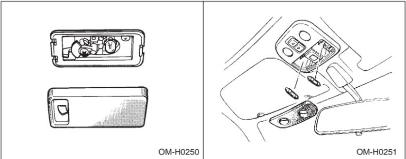
1. Remove the lens by prying the edge of the lens with a regular screwdriver.
