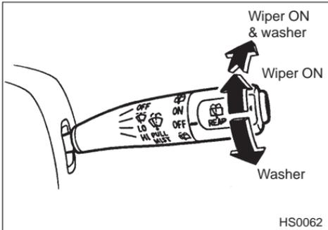
To turn the rear wiper on, turn the knob on the end of the wiper control lever to the “ON” position.
