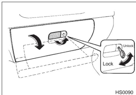
To open the glove compartment, pull the handle. To close it, push the lid firmly upward.
