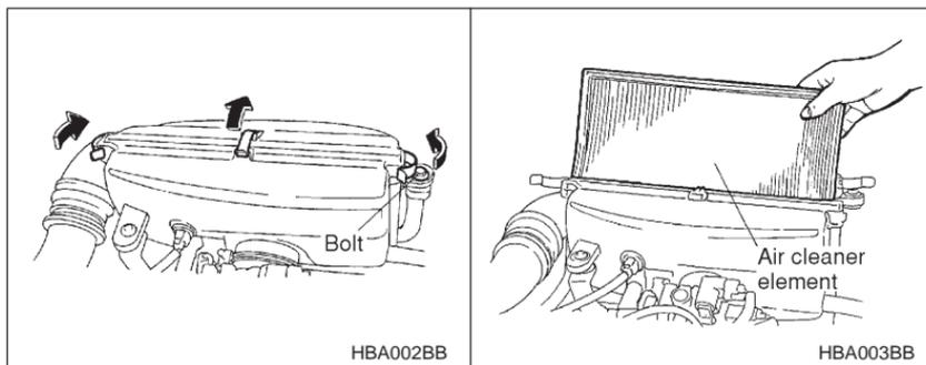
1. Remove the bolt securing the rear air cleaner element case.
