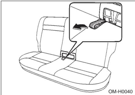
4. Unlock the seatback by pulling the release knob and fold it down. Confirm that the pin located at the bottom of the seat cushion is inserted into the slot at the top of the seatback.
