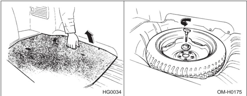
The spare tire is stored under the floor of the trunk or the luggage compartment. To remove the spare tire, first remove the spare tire cover, turn the attaching bolt counterclockwise, then take the spare tire out.
