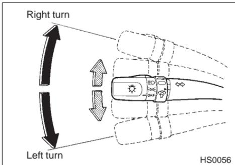
To activate the right turn signal, push the turn signal lever up. To activate the left turn signal, push the turn signal lever down. When the turn is finished, the lever will return automatically. If the lever will not return after cornering, return the lever to the neutral position by hand.
