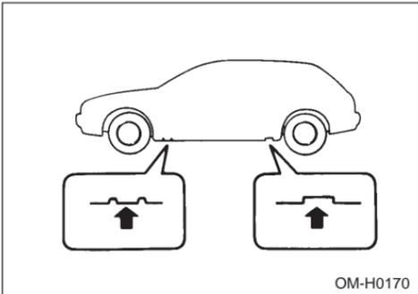
9. Insert the jack handle into the jackscrew, and turn the handle clockwise until the tire clears the ground. Do not raise the vehicle higher than necessary.
