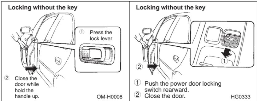
To lock the door from the outside without the key, press the end of the lock lever down on the door and then close the door.
