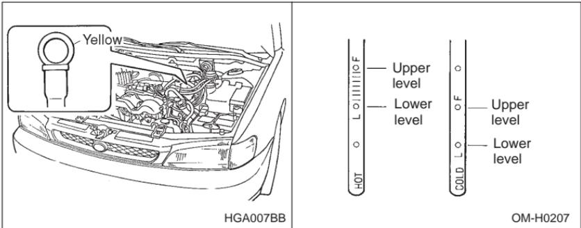
4. Pull out the dipstick and check the fluid level on the gauge. If it is below the lower level on the “HOT” range, add the recommended automatic transmission fluid up to the upper level.
