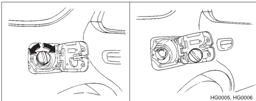
To take off the fuel filler cap, turn it slowly counterclockwise and remove the cap. While refueling, hang the cap on the cap holder inside the fuel lid.
