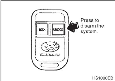
To disarm the system, press and release the “UNLOCK” button. The siren will chirp and parking lights will flash **once**. The driver's door will unlock at this time, and the vehicle interior (dome) light will turn on for 60 seconds, or until the vehicle is started.
