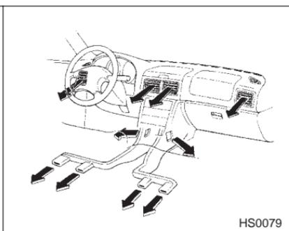
This setting allows you to direct air of different temperatures from the instrument panel and outlets. The air from the foot outlets is slightly
