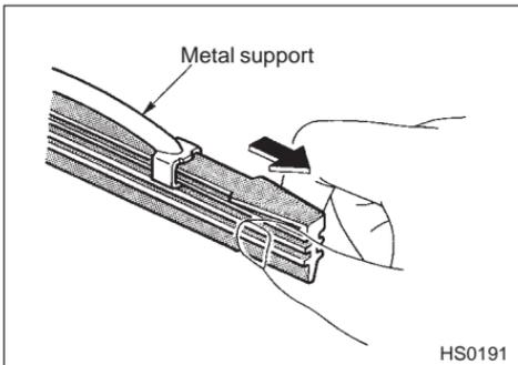
4. If the new blade rubber is not provided with two metal spines, remove the metal spines from the old blade rubber and install them in the new blade rubber.
