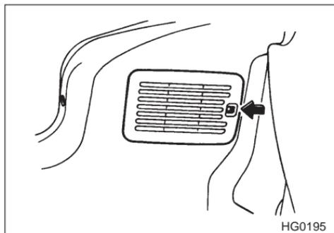
1. Unlatch the rear combination light cover by pulling the knob. Open the cover up.
