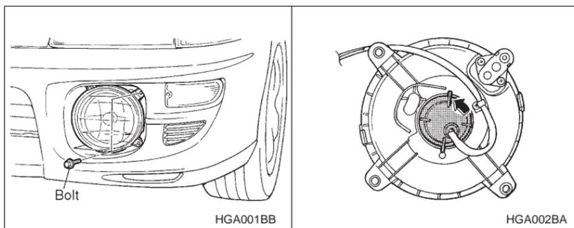
1. Remove the front fog light assembly by removing the three bolts.
