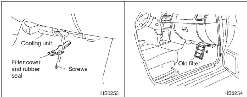
1. Remove the filter cover by removing the two (2) screws.
