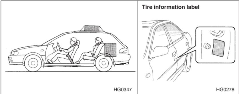
The load capacity of your vehicle is determined by weight, not by available cargo space. The maximum load you can carry in your vehicle is shown as the Vehicle Capacity Weight on the tire information label attached to the driver's side door jamb. It includes the total weight of driver and all passengers and their belongings, any optional equipment such as a trailer hitch, roof rack or bike carrier, etc., and the tongue load of a trailer.
