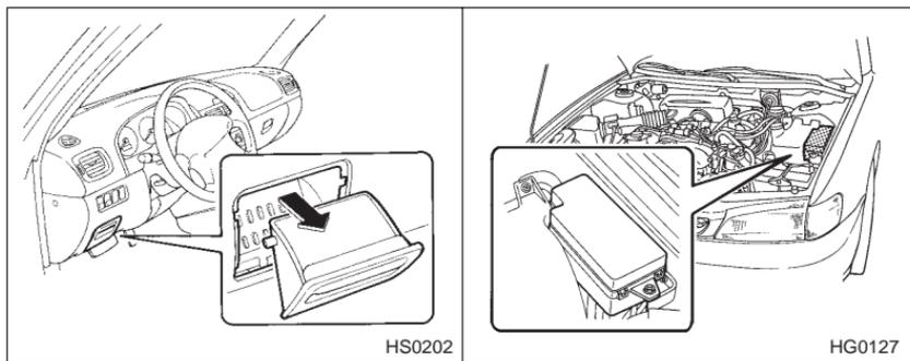
The fuses are designed to melt during an overload to prevent damage to the wiring harness and electrical equipment. The fuses are located in two fuse boxes.
