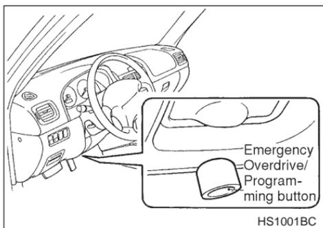
The Emergency Override/Programming button is used to disarm the alarm system in case of a lost or broken transmitter. It is also used in conjunction with the transmitter and vehicle ignition to program additional transmitters.
