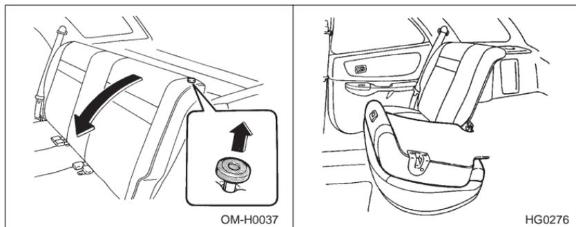
Unlock the seatback by pulling the release knob and fold it down.
