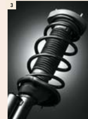
3 The new 2.5 XS L.L.Bean Edition offers an exclusive, self-leveling rear suspension that helps keep the vehicle level regardless of load.
