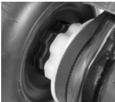
Figure 3c. Align the power coupling and tighten until the axle is tight against the frame.
