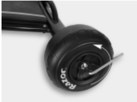
Figure 3e. Tightening the backwards threaded axle.
