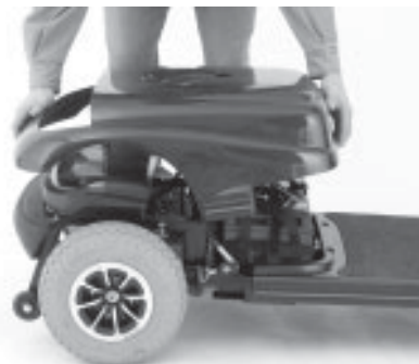
Figure 19. Rear Shroud Removal
