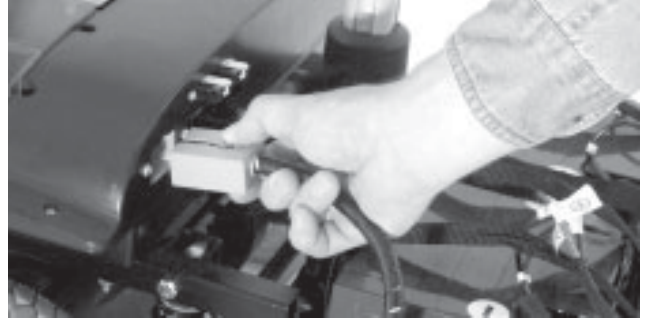
Figure 21. Disconnecting The Front-To-Rear Harness
