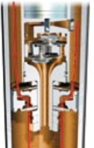
Rebound in 'Sport' mode – working piston only, sporty-hard tuning
