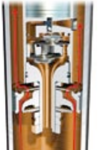
Compression in 'Sport' mode – working piston only, sporty-hard tuning
