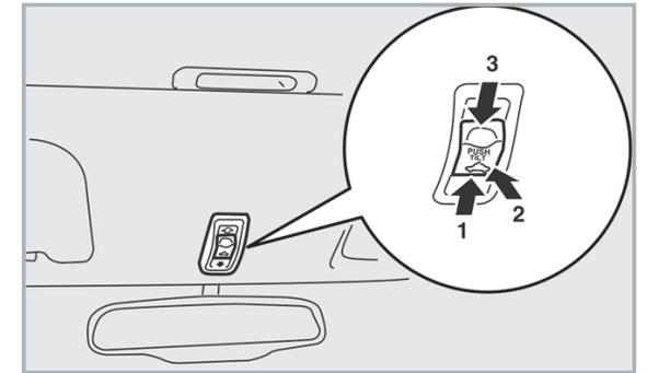
Press the switch **3**, and the sunroof will close while the switch is pressed.
