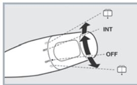
operates intermittently at intervals of about eight seconds. You can adjust the intervals of the operation by using the multi-center display (if equipped).
