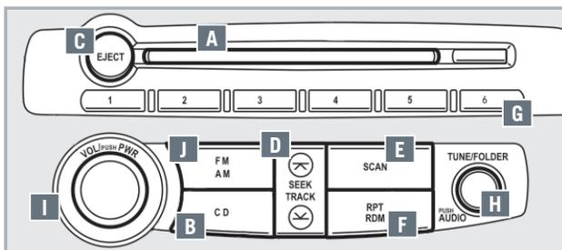
Press the LOAD/EJECT button **C**, then press one of the disc select buttons **G** to select the slot where you wish to eject the disc.
