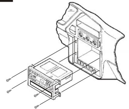
Re-connect the battery terminal and test the unit for proper operation. Mount the head unit/kit assembly to the sub-dash with (4) screws previously removed in step #1.
