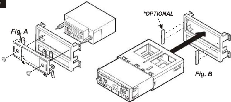
**2-SHAFT HEAD UNITS:** Attach the *Faceplate* to the *Radio Housing*. Slide the aftermarket head unit into the kit and secure with shaft nuts. (see Fig. A)
