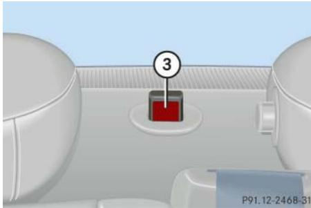
If the backrest is not locked into position, a red indicator ③ will be visible.
