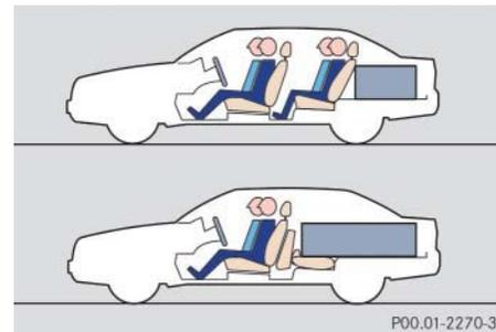
The total load weight including vehicle occupants and luggage/cargo should not exceed the vehicle capacity weight indicated on the corresponding label located on the driver's door pillar.
