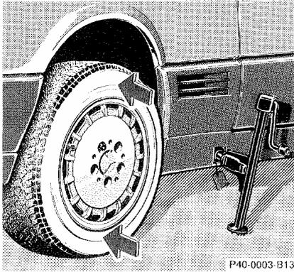
10. Clean contact surfaces of wheel and wheel hub. Install spare wheel on wheel hub. Insert wheel bolts and tighten them slightly.
