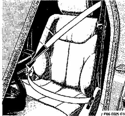
Adjust seat belt so that shoulder portion is located as close as possible to the middle of your shoulder. Do not twist the belt.
