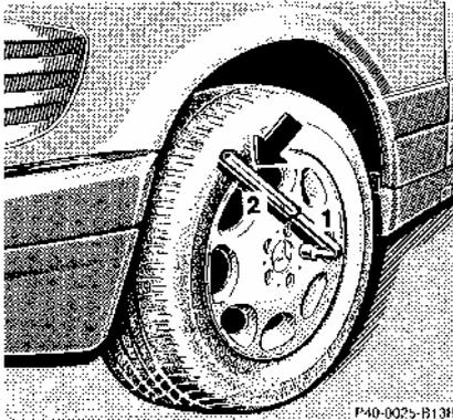
6. Remove lug wrench (1) and extension (2) from tool kit and assemble. Loosen but do not yet remove the wheel bolts.
