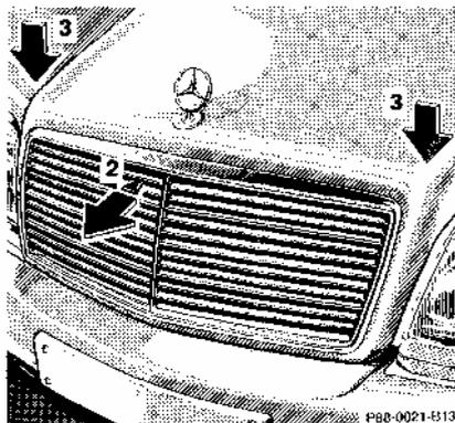
Pull handle (2) out of radiator grill to stop and open hood. Do not lift hood at louvers of grill! Make certain the windshield wiper arm is not folded forward.
