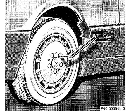
12. Using the wrench, tighten the five bolts evenly, following the sequence illustrated above, until all bolts are tight.
