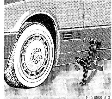
7. Jack up the vehicle until the wheel is clear of the ground. Never start engine while vehicle is raised.
