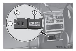
The 115 V AC power socket ① provides an alternating voltage of 115 V, so that small electronic devices can be connected. These devices, such as games consoles, chargers and laptops, should not consume more than a maximum of 150 W altogether.
