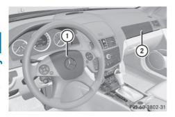
Driver's air bag (1) deploys in front of the steering wheel; front-passenger air bag (2) deploys in front of and above the glove box. They are deployed:
