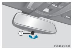
► Anti-glare mode: flick anti-glare switch (1) forwards or back.
