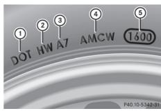
The TIN is a unique identification number. The TIN enables the tire manufacturers to inform purchasers of recalls and other safety-relevant matters. It makes it possible for the purchaser to easily identify the affected tires. The TIN is made up of manufacturer identification code (2), tire size (3), tire type
