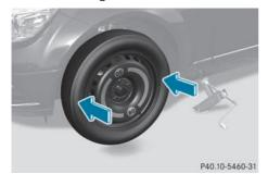
▶ Place the emergency spare wheel on the wheel hub and push it on.
