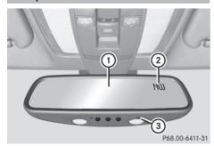
To obtain correct direction display in rearview mirror ①, the compass must be calibrated and the magnetic field zone set.
