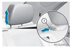
If the head restraint is fully lowered, it is necessary to press release catch (1).
