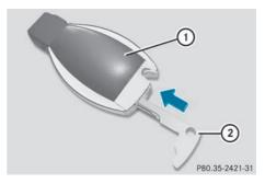
▶ Press mechanical key ② into the opening in the SmartKey in the direction of the arrow until battery tray cover (1) opens. Do not hold the cover closed while doing so.
