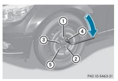
▶ Tighten the wheel bolts evenly in a crosswise pattern in the sequence indicated (1) to (5)). The tightening torque must be 96 lb-ft (130 Nm).
