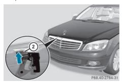
▶ Reach into the gap, pull hood catch handle ② up and lift the hood.
