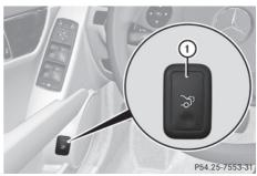
▶ To open: press the upper section of remote operating switch (1) for the trunk lid until the trunk lid opens.
