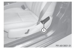
Pelvis air bags (1) deploy next to and below the outer seat cushions. They are deployed:
