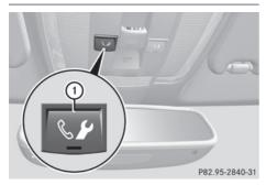
▶ Press and hold Roadside Assistance button ① for more than two seconds. A call to a Mercedes-Benz Roadside Assistance Representative is initiated. The indicator lamp in Roadside Assistance button ① flashes while the call is active. The Connecting Call message appears in the multifunction display and the audio system or COMAND is muted.
