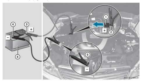
Position number (6) identifies the charged battery of the other vehicle or an equivalent jump-starting device.
