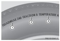
The Uniform Tire Quality Grading Standards are U.S. government specifications. Their purpose is to provide drivers with uniform reliable information on tire performance data. Tire manufacturers have to grade tires using three performance factors: (1) tread wear, (2) tire traction, and (3) heat resistance. All tires sold in North America are provided with the corresponding quality class mark on the sidewall of the tire, even though these regulations do not apply to Canada.
