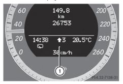
▶ Shift gear according to the gearshift recommendation (1) shown in the multifunction display of the instrument cluster.
