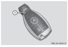
▶ Press the 🕡 or 🕡 button. The SmartKey battery is working properly if battery charge indicator lamp (1) lights up briefly.
