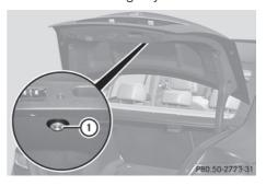
The trunk lid can be unlocked and opened with the trunk lid emergency release when the vehicle is stationary or while driving.
