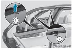
► To extend: pull the roller sunblind out by tab ① and hook it onto retainers ② at the top of the window.
