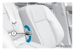
Move adjustment lever ① in the direction of the arrow until the desired backrest contour is achieved.
