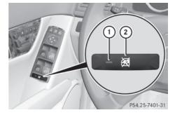
▶ To activate/deactivate: press button ②. If indicator lamp (1) is lit, operation of the rear side windows is disabled. Operation is only possible using the switches in the driver's door. If indicator lamp (1) is off,
