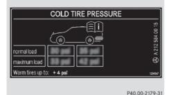
Tire pressure table for all approved tires installed at the factory (example)
