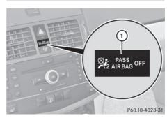
Special child restraint systems which are compatible with BabySmart<sup>TM</sup> are necessary for deactivating the front-passenger front air bag. When the special child restraint system which is compatible with BabySmart<sup>TM</sup> is installed correctly and is recognized by the sensor system in the front-passenger seat, the front-passenger front air bag is deactivated. In this case,
