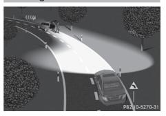
The active light function is a system that moves the headlamps according to the steering movements of the front wheels. In this way, relevant areas remain illuminated while driving. This allows you to recognize pedestrians, cyclists and animals.
