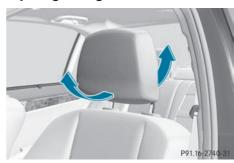
▶ Push or pull the lower edge of the head restraint in the direction of the arrow.
