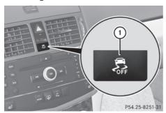
▶ To activate: briefly press button ①. The SPORT warning lamp in the instrument cluster lights up. The SPORT handling
