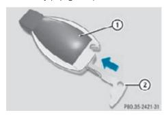
▶ Press mechanical key (2) into the SmartKey opening until battery compartment cover (1) opens. Do not keep the cover shut.
