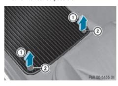
▶ **Removing:** Pull floormat off of retainer pins (2) in direction of arrow (1).
