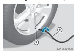
► Unscrew the valve cap of the damaged tire from tire valve (9).
