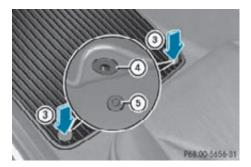
▶ **Installing:** Press floormat eyelets ④ onto retainer pins ⑤ in direction of arrow ⑥.
