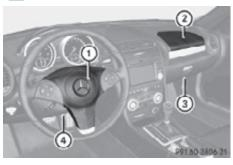
Driver's front air bag ① and passenger front air bag ② are designed to provide increased protection for the driver and passenger against the risk of injuries to the head and thorax.
