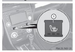
The red indicator lamps in seat heating switch ① come on to show which heating level you have selected.
