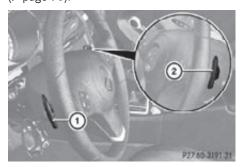
Steering wheel gearshift control (example illustration)
