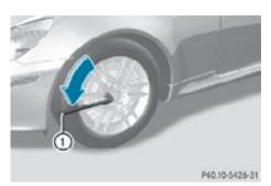
► On the wheel to be changed, loosen but do not yet remove the wheel bolts (approximately one full turn with wheel wrench (1)).
