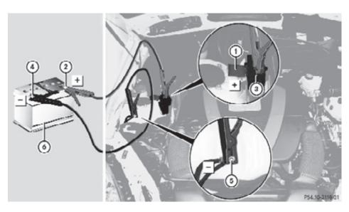
Position (6) represents the charged battery of another vehicle or an equivalent starter pack.
