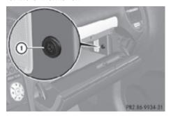
AUX socket ① is designed for a 3.5 mm stereo jack (3-pin), for devices with dedicated analog audio output or connection via headphone port, e.g. MP3 or tape player.
