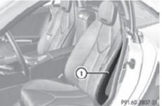
Head-thorax air bags ① are designed to provide increased protection for the head and thorax but not for the arms.
