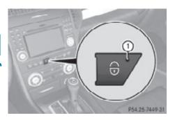
► **Arming:** Lock the vehicle with the SmartKey.
