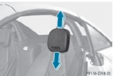
► Adjust the height of head restraints manually by pulling them upwards or pushing them downwards.
