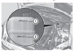
The brake fluid level is correct when it is between lower mark (MIN) ② and upper mark (MAX) ① of the brake fluid reservoir.
