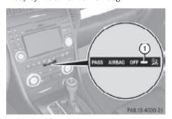
PASS AIR BAG OFF [ indicator lamp 1 will be illuminated, except with the SmartKey removed from the starter switch or with the starter switch in position 0.
