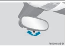
► Tilt the mirror to the antiglare position by moving lever towards the windshield.
