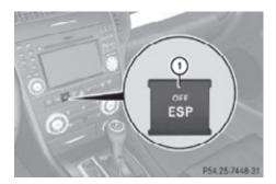
► With the engine running, press ESP® switch ① until the ESP® warning lamp
