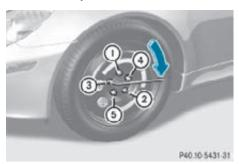
➤ Tighten the five wheel bolts evenly, following the diagonal sequence illustrated (1) to (5), until all bolts are tight. Observe a tightening torque of 80 lb-ft (110 Nm).
