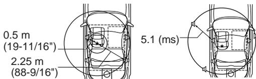
Here we calculate the time correction value for the front right tweeter in the diagram at the left.
