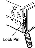
Slide the CDA-7969/CDA-7867 into the dashboard. When the unit is in place, make sure the locking pins are fully seated in the down position. This can be done by pressing firmly in on the unit while pushing the locking pin down with a small screwdriver. This ensures that the unit is properly locked and will not accidentally come out from the dashboard.
