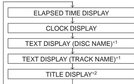
\*1 Displayed during playback of a text compatible CD (when using an optional text compatible). "NO TEXT" will be displayed when the CD is not text compatible.
