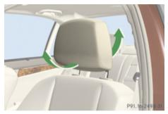
Adjust the head restraint to the desired position by pushing or pulling on the lower edge of the head restraint cushion.
