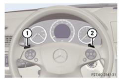
Steering wheel gearshift control (example illustration)
