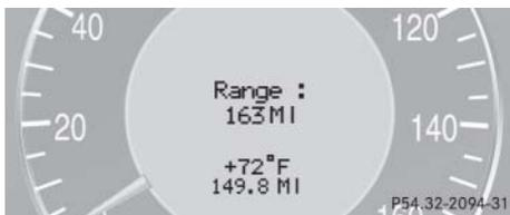
**i** If only very little fuel is left in the tank, a vehicle at the fuel pump is shown instead of the range.
