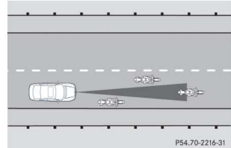
Because of their narrow profile, the vehicles traveling near the outer edges of the lane have not yet been detected by DISTRONIC. There will be insufficient distance to the vehicles ahead.
