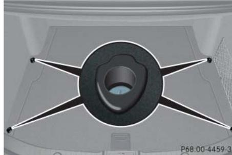
► Carefully secure cargo by applying even load on all hooks with rope of sufficient strength to hold down the cargo.
