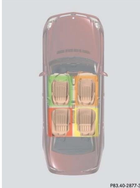
With the help of a sun sensor, the climate control determines the relation of the sun to the vehicle and automatically adjusts the inside temperature for every individual zone.
