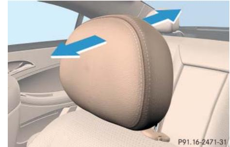
Manually adjust the head restraint.
