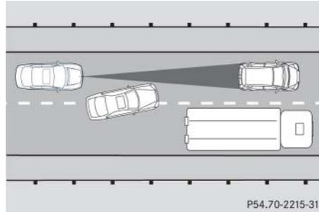
DISTRONIC has not yet detected the vehicle changing lanes. There will be insufficient distance to the lane-changing vehicle.
