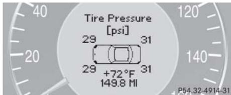
**i** When the vehicle has been parked for longer than 20 minutes, the message Tire pressure is only displayed after driving for a few minutes. *appears in the multifunction display.*
