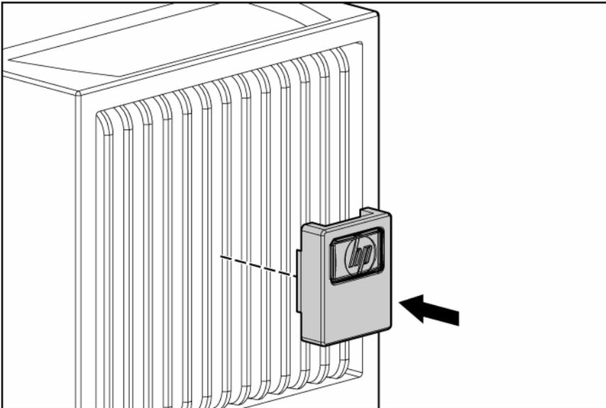
3. From inside the bezel, gently push out the LED/Control panel and rotate 90 degrees.
