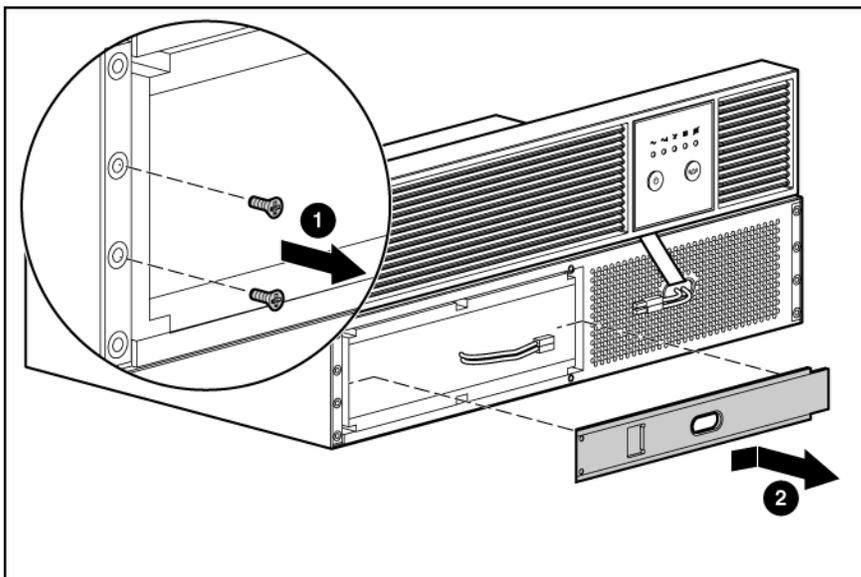
5. Remove the UPS battery modules.
