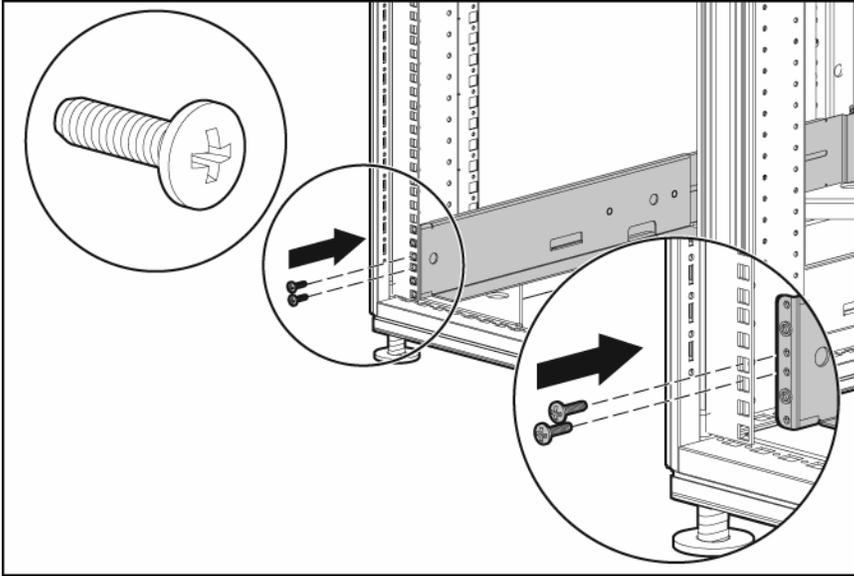
4. Insert screws through the rack into the mounting rail and the rear of each mounting bracket. Do not completely tighten the screws.
