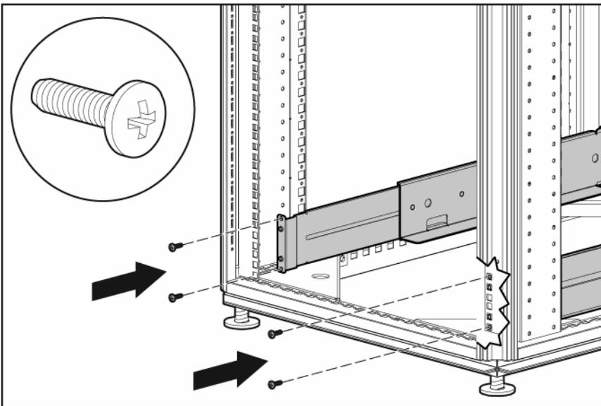
5. Wait until the unit is installed and the brackets are adjusted before tightening the screws.
