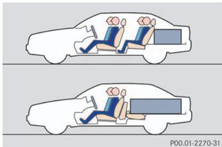
The total load weight including vehicle occupants and luggage/cargo should not exceed the vehicle capacity weight indicated on the certification tag which can be found on the left door pillar.
