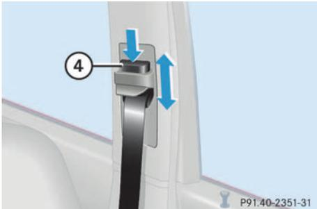
**4** Button for belt outlet height adjustment
