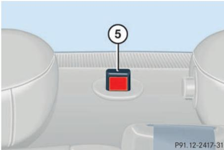
If the backrest is not locked into position, a red indicator **5** will be visible.
