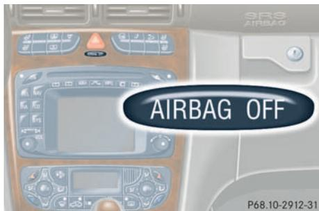
Special BabySmart™ compatible child seats, designed for use with the Mercedes-Benz system and available at any authorized Mercedes-Benz Center are required for use with the BabySmart™ airbag deactivation system. With the special child seat properly installed, the passenger front airbag will not deploy.
