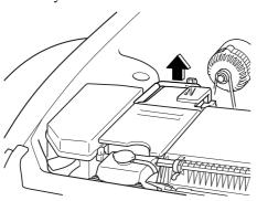
3. Remove the battery cover from its rear side.
