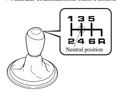
The shift pattern of the transmission is conventional, as shown.
