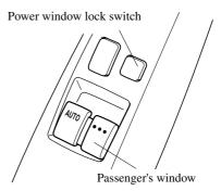
To open the window to the desired position, hold down the switch. To close the window to the desired position, pull up the switch.
