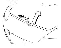
3. Grasp the support rod and secure it in the stay hole indicated by the arrow to hold the hood open.
