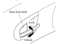
To lock either front door with the door-lock knob from the outside, push the door-lock knob to the lock position and close the door.
