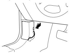
3. Pull the fuse straight out with the fuse puller provided on the inside of the engine compartment fuse block cover.
