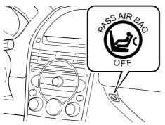
If the front passenger weight sensors are working properly, the indicator light illuminates when the ignition switch is turned to the ON position. After about 6 seconds it goes out.
