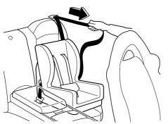
3. Push the child-restraint system firmly into the vehicle seat. Be sure the belt retracts as snugly as possible. Clicking from the retractor will be heard during retraction if the system is in the automatic locking mode. If the belt does not lock the seat down tight, repeat this step.
