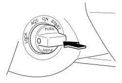
7. Verify that the KEY indicator light (green) illuminates in the instrument cluster. The KEY warning light (red) means you cannot continue to start the engine (page 3-21).
