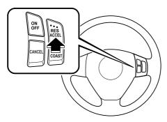
Your vehicle has a tap-up feature that allows you to increase your current speed in increments of 1.6 km/h (1 mph) by a momentary tap of the RES/ACCEL button. Multiple taps will increase your vehicle speed 1.6 km/h (1 mph) for each tap.
