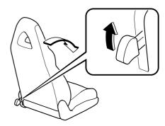
To return it to the upright position, lift the seatback and push it into place. Rock the seatback to make sure it is locked.
