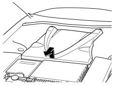
2. Remove the rubber hose from the battery cover.
