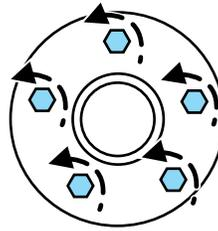
6. Loosen each wheel lug nut one-half turn counterclockwise but do not remove them until the wheel is raised off the ground.
