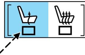
The heated seat module resets at every ignition run cycle. While the ignition is in the on position, activating the high or low heated seat switch enables heating mode. When activated, they will turn off automatically when the ignition is turned to the off position.
