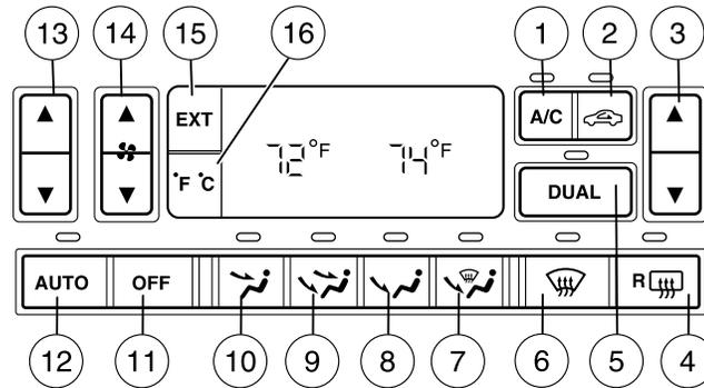
1. **A/C control:** Cools the vehicle and is used to reduce humidity in the vehicle. Press to turn on/off.
