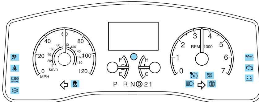
Warning lights and gauges can alert you to a vehicle condition that may become serious enough to cause expensive repairs. A warning light may illuminate when a problem exists with one of your vehicle's functions. Many lights will illuminate when you start your vehicle to make sure the bulb works. If any light remains on after starting the vehicle, refer to the respective system warning light for additional information.
