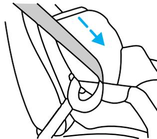
6. Allow the belt to retract to remove slack. The belt will click as it retracts to indicate it is in the automatic locking mode.
