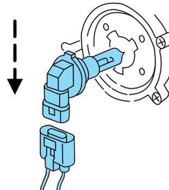
**!** **WARNING:** Handle a halogen headlamp bulb carefully and keep out of children's reach. Grasp the bulb only by its plastic base and do not touch the glass. The oil from your hand could cause the bulb to break the next time the headlamps are operated.
