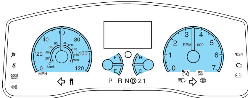
**Speedometer:** Indicates the current vehicle speed. Refer to the *Message center* in this chapter to change your display to a digital speedometer. The digital display is more accurate than the analog gauge and may not match.
