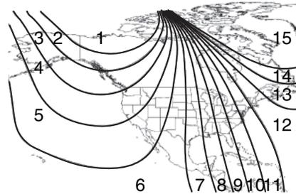
6. Press the SELECT control repeatedly until the correct zone setting for your geographic location is displayed on the message center. The range of zone values are from 01 to 15 and “wraps” back to 01.
