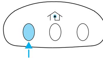
2. Simultaneously press and hold both the chosen HomeLink® and hand-held transmitter buttons until the HomeLink® indicator light changes from a slow to a rapidly blinking light. Now you may release both the HomeLink® and hand-held transmitter buttons.
