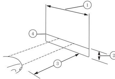
3. Turn on the low beam headlamps to illuminate the wall or screen and open the hood.
