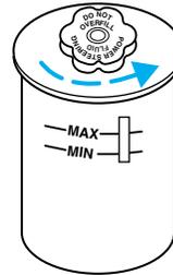
5. If the fluid is low, add fluid in small amounts, continuously checking the level until it reaches the range between the MIN and MAX lines. Be sure to put the cap back on the reservoir. Refer to *Maintenance product specifications and capacities* in this chapter for the proper fluid type.
