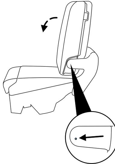
**!** **WARNING:** Ford Motor Company recommends that all front seat armrests should be inspected by an authorized dealer after any collision to verify that the locking pin feature has not been damaged. The front seat armrest must be replaced if either damage or improper operation is found. Failure to replace a damaged front seat armrest may result in the armrest falling suddenly during a collision, which could lead to serious injury.
