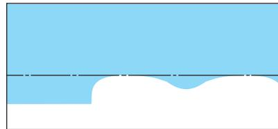
To see a clearer light pattern for adjusting, you may want to block the light from one headlamp while adjusting the other.
