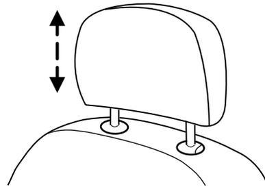
Push control to lower head restraint.
