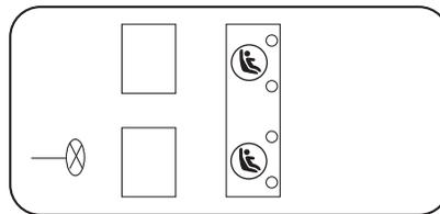
The LATCH anchors are located at the rear section of the rear seat between the cushion and seatback, below the locator symbols on the seat back. Follow the child seat manufacturer's instructions to properly install a child seat with LATCH attachments.
