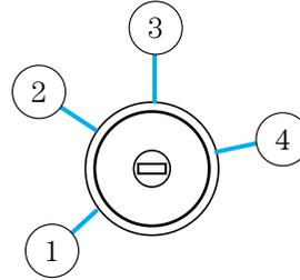
If the key has been successfully programmed it will start the vehicle's engine and the theft indicator light will illuminate for three seconds and then go out. If the key was not successfully programmed, it will not start your vehicle's engine and the theft indicator light will flash on and off rapidly. If failure repeats, bring your vehicle to your authorized dealer to have the new key(s) programmed.
