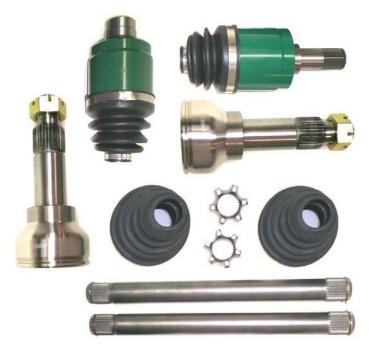
**Step 1:** Assemble Small end of axle shaft with the Mini cv joint assembly as done on a stock Mini but replace ball bearing gear with supplied gear.
