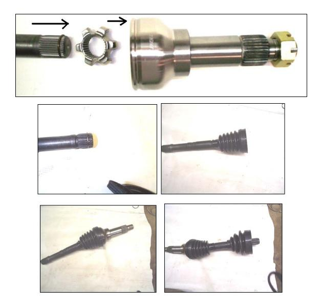
**Honda Axle End Assembly:** Assemble large splinned side of axle with the Honda cv joint assembly. (See following four Photos)
