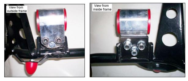
**Step 4:** Attach MTK engine mounting bracket to engine block as shown. For some engines, you will need to use the supplied spacer plates for clearance.
