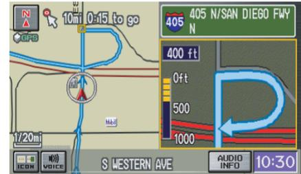
On the map screen, the location of the maneuver is marked with a small yellow square. The guidance window is simply an enlargement of the area indicated by the yellow square. After you complete the maneuver, the display returns to a full map screen when the single-screen mode is set, or to a map and direction list screen when the split-screen mode is set.
