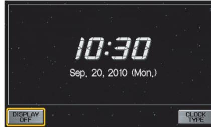
If you are not planning to use the navigation system at this time, touch **DISPLAY OFF** to turn off the screen.
