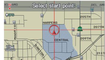
Use the **ZOOM** buttons to select the map scale (available scales are 1/20, 1/8, and 1/4 mile scales). Use the joystick to move the crosshairs (red circle) to the desired start point and push in the joystick to “set” the start point. Then move the joystick in a straight or diagonal direction to encompass the area to be avoided.
