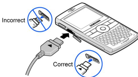
2. Plug the adaptor into a standard AC wall outlet. When charging is finished, unplug the adaptor from the power outlet.
