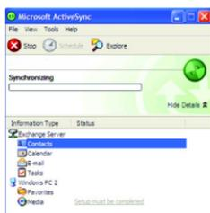
Once the synchronization is completed, the phone stays connected to the computer. If any change is made, Microsoft® ActiveSync® automatically will begin synchronization. To begin synchronization, press the **Sync** soft key in Microsoft® ActiveSync® on your phone. You can open the phone's file directory by clicking **Explore** from the Microsoft® ActiveSync® window. You can then copy files quickly and easily from the phone to the computer, or vice versa.
