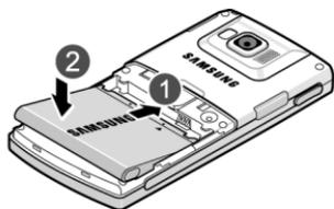
3. With the battery in position on the phone, place the cover back on the handset and slide it in until it clicks.
