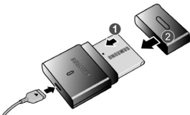
2. Plug the power cord into the wall outlet after you have inserted the battery into the battery charger and closed the lid.
