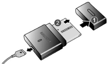
3. Once the battery has completed charging, unplug the cord from the wall outlet, open the battery charger, and remove the charged battery from the charger.
