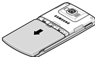
2. Remove the battery cover by pressing the battery lock down and slide the battery cover away, as shown.
