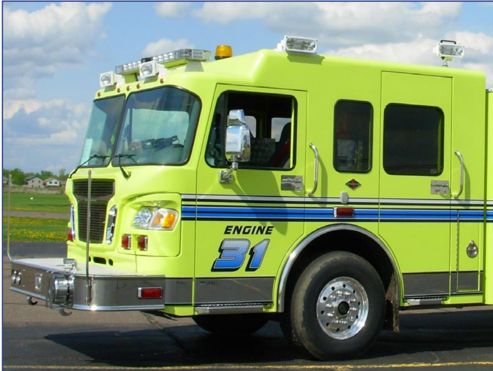
Above: Spartan custom cab mount and Magnafire 3000® HID floodlight Model shown: KR-1539-SP-KOV
