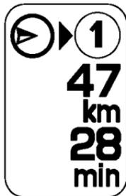
The distance and time to destination symbol indicates the distance and the estimated time remaining to the final destination, depending on the option selected.
