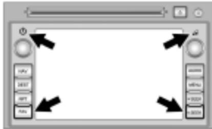
6. To close the screen, slightly push up on the two outer corners until the screen is in position. Then push the screen in by pushing on the four outer corners until a click is heard.
