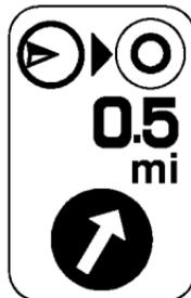
The straight line to distance symbol indicates the straight-line distance to the destination.
