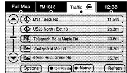
1. Press the NAV key, then press the NAV key repeatedly until Traffic is selected, or touch the Traffic screen button. A list of traffic conditions may display with the direction and how far away the traffic conditions are from the vehicle's current position.
