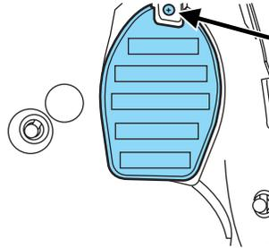
4. From the exterior wheel well area, reach arm through splash shield opening to access bulb socket (Passenger side only).
