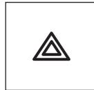
Push in the flasher control and all front and rear direction signals will flash. Press the flasher control again to turn them off. Use it when your vehicle is disabled and is creating a safety hazard for other motorists.
