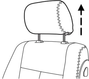
2. Simultaneously press and hold both the adjust/release button and the unlock/remove button, then pull up on the head restraint.
