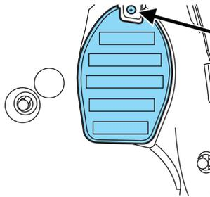
5. From the exterior wheel well area, reach arm through splash shield opening to access bulb socket (Passenger side only).
