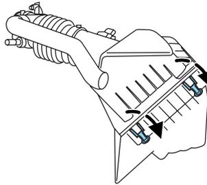
1. Release the clamps that secure the air filter housing cover.
