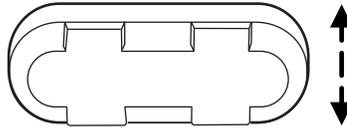
Press the switch in the direction of the arrows to move the seat forward, backward, up or down.
