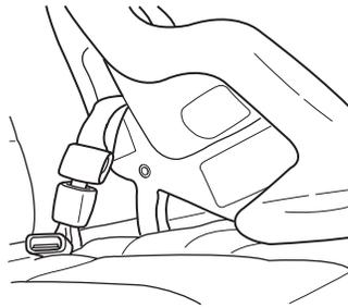
Airbags can kill or injure a child in a child seat. NEVER place a rear-facing child seat in front of an active airbag. If you must use a forward-facing child seat in the front seat, move the vehicle seat all the way back.
