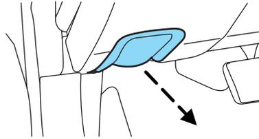
2. Go to the front of the vehicle and release the auxiliary latch that is located under the front center of the hood.
