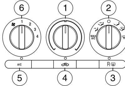
**MAX A/C:** Distributes recirculated air through the instrument panel vents only to cool the vehicle. This re-cooling of the interior air is more economical and efficient. Recirculated air may also help reduce undesirable odors from entering the vehicle.
