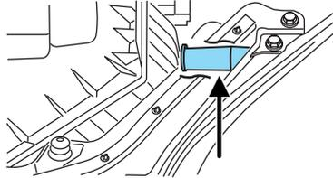
4. Remove screw from oval splash shield access panel from the exterior wheel well area. Lift up and rearward to release a hidden finger attachment at the lower portion of the panel (Passenger side only).
