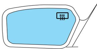
**Do not remove ice from the mirrors with a scraper or attempt to readjust the mirror glass if it is frozen in place.**
