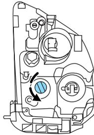
6. Let go of the bulb socket and let the bulb socket dangle downward near the lamp housing (Passenger side only).
