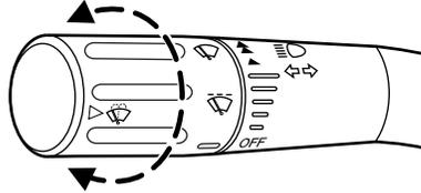
**Speed dependent wipers:** When the wiper control is set on the intermittent settings, the speed of the wipers will automatically adjust with the vehicle speed. The faster your vehicle is travelling the faster the wipers will go.
