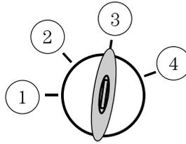
**Note:** If the engine does not start on the first try, turn the key to the off position, wait 10 seconds and try step 2 again. If the engine still fails to start, press the accelerator to the floor and try step 2 again, keeping the accelerator on the floor until the engine begins to accelerate above cranking speeds; this will allow the engine to crank with the fuel shut off in case the engine is flooded with fuel.
