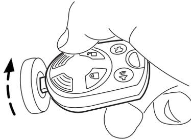
Likewise, when rotating the IKT to the off position in the ignition lock cylinder, the bottom edge of the IKT adjacent to the
