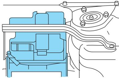
**If your battery has a cover/shield, make sure it is reinstalled after the battery has been cleaned or replaced.**
