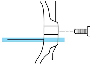
7. Add enough fluid through the filler opening so that the fluid level is within 3/8 inch (10mm) of the bottom of the filler hole with the vehicle on a level surface.
