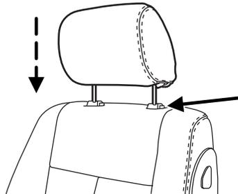
Properly adjust the head restraint so that the top of the head restraint is even with the top of your head and positioned as close as possible to the back of your head. For occupants of extremely tall stature, adjust the head restraint to its full up position.
