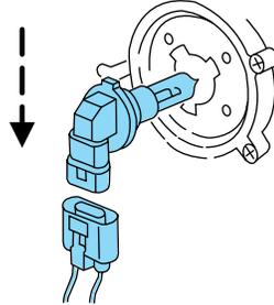
12. After the new bulb is installed, carefully let the bulb socket dangle downward near the lamp housing (Passenger side only).
