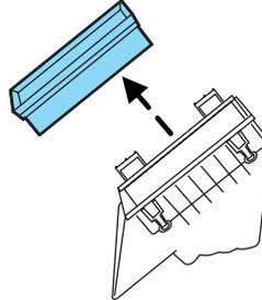
3. Remove the air filter element from the air filter housing.
