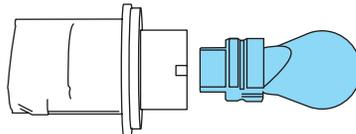
10. From the exterior wheel well area reach arm through splash shield opening to install bulb socket with new bulb (Passenger side only).
