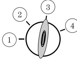
1. Insert the first previously programmed **coded key** into the ignition.
