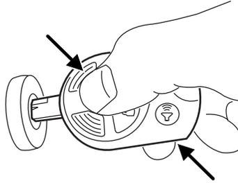
To gain more leverage when rotating the IKT in the ignition lock cylinder, you can readjust the location of your thumb to grasp the IKT on the outer edge next to the
