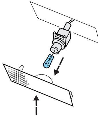
4. With the bulb exposed, carefully remove the bulb from the socket by grasping the bulb and pulling it away from the wire harness. Replace with a new bulb, and reverse the removal steps to complete the process.
