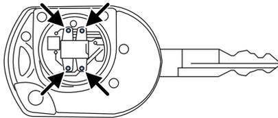
3. Remove the old battery. **Note:** Please refer to local regulations when disposing of transmitter batteries.
