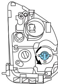
6. Carefully pull bulb straight out of socket and push in the new one.
