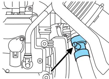
5. Open the coolant bleed valve on the back of the engine water outlet for the 2.3L engine or the coolant bleed valve located on the upper radiator hose for the 3.0L engine.
