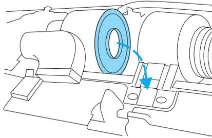
5. Install a new air filter element. Be careful not to crimp the filter element edges between the air filter housing. This could cause filter damage and allow unfiltered air to enter the engine if not properly seated.
