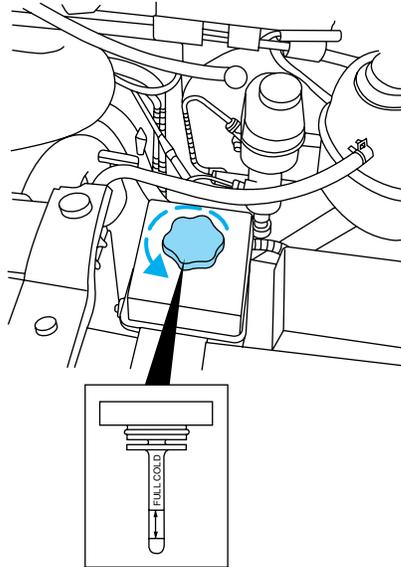
Check the fluid level when it is at ambient temperature, 20° – 80° F (-7° – 25° C):
