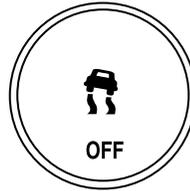
The AdvanceTrac® with RSC system warning indicator light may flash to indicate the system is not fully initialized. If this happens, slow down. If the light continues flashing, have the AdvanceTrac® with RSC system serviced by an authorized dealer.
