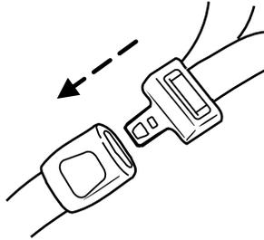
2. To unfasten, push the release button and remove the tongue from the buckle.
