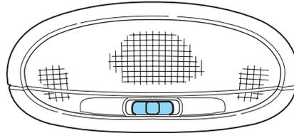
When the control is in the OFF position, it will not illuminate when you open the doors or fully rotate the headlamp control.
