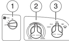
**VENT:** Distributes outside air through the instrument panel vents.
