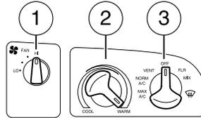
**MAX A/C:** Uses recirculated air to cool the vehicle. Air flows from the instrument panel vents only.
