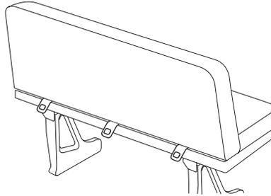
3. Clip the tether strap hook to the tether bracket mounted under rear rail of seat cushion frame.
