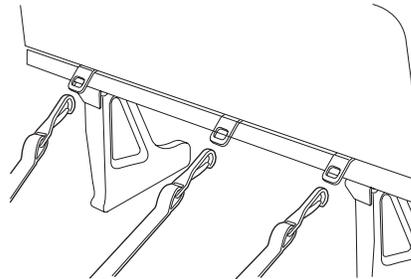
4. Install the child safety seat tightly using the LATCH anchors or safety belts. Follow the instructions in this chapter.
