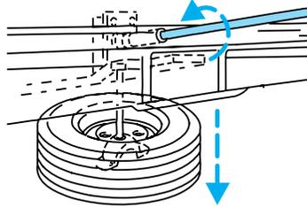
To stow the cable retainer with the spare removed, turn the jack handle clockwise until all slack is removed.
