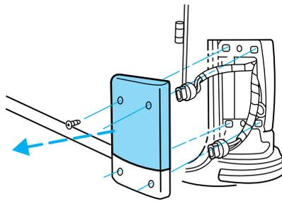
2. Rotate bulb socket counterclockwise and remove from lamp assembly.
