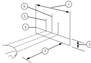
2. The center of the headlamp is marked either on the lens (a circle or cross marker) or on the bulb shield, internal to the lamp (mark or feature). Measure the height from the center of your headlamp to the ground (2) and mark an 8 foot (2.4 meter) long horizontal line on the wall or screen (1) at this height (masking tape works well).
