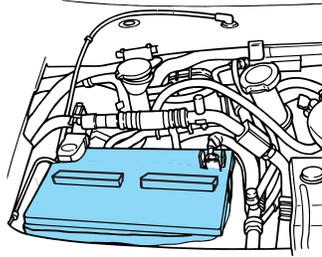
**If your battery has a cover/shield, make sure it is reinstalled after the battery has been cleaned or replaced.**
