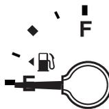
The FUEL icon and arrow indicates which side of the vehicle the fuel filler door is located.
