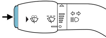
**Note:** Do not operate the washer when the washer reservoir is empty. This may cause the washer pump to overheat. Check the washer fluid level frequently. Do not operate the wipers when the windshield is dry. This may scratch the glass, damage the wiper blades and cause the wiper motor to burn out. Before operating the wiper on a dry windshield, always use the windshield washer. In freezing weather, be sure the wiper blades are not frozen to the windshield before operating the wipers.
