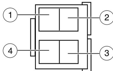
The instrument panel relay module is located behind the radio in the center of the instrument panel. Have your authorized dealer service this module, if required.
