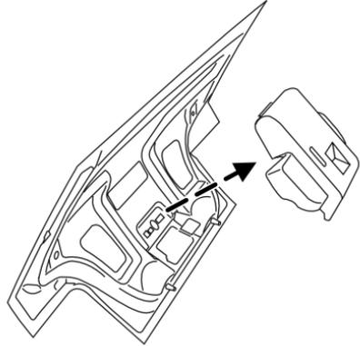
4. Carefully pull the bulb straight out of socket.
