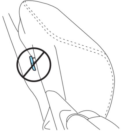
4. Access tether anchors located behind the seatback under the vinyl tag marked with the child tether anchor symbol.
