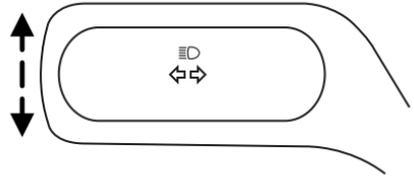
The flash rate of the turn signal will speed up considerably if the Lighting Control Module detects a left or right turn lamp bulb (front or rear) is burned out.
