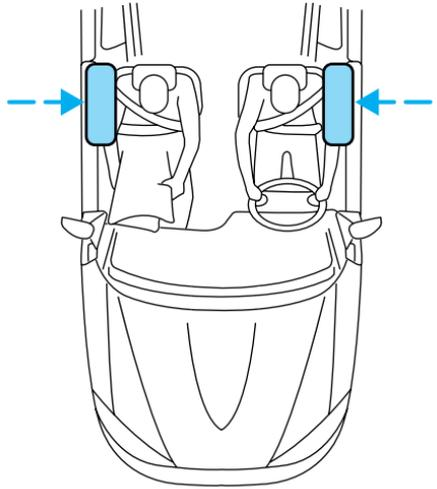
Side airbags, in combination with safety belts, can help reduce the risk of severe injuries in the event of a significant side impact collision.
