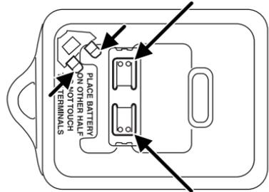
3. Remove the old battery. **Note:** Please refer to local regulations when disposing of transmitter batteries.
