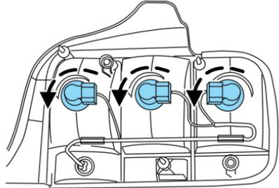
5. Remove the bulb socket by rotating it counterclockwise, then pulling it out of the lamp assembly.
