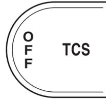
If you should become stuck in snow or ice or on a very slippery road surface, try switching the Traction Control™ system off. This may allow excess wheel spin to “dig” the vehicle out and enable a successful “rocking” maneuver.
