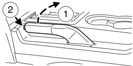
The BRAKE warning lamp will illuminate and will remain illuminated until the parking brake is released.
