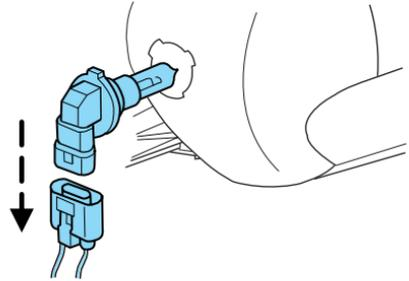
5. Rotate the bulb counterclockwise and remove from the lamp assembly.
