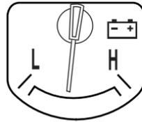
**Engine oil pressure gauge (if equipped):** Indicates engine oil pressure. The needle should stay in the normal operating range (between "L" and "H"). If the needle falls below the normal range, stop the vehicle, turn off the engine and check the engine oil level. Add oil if needed. If the oil level is correct (and gauge reads no/low oil pressure....), shut down the engine immediately and contact your dealer for service or by a qualified technician.
