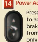
Press and hold the rocker control to adjust the accelerator and brake pedal toward you or away from you. Adjust the pedals only when the vehicle is stopped and the gearshift lever is in the P (Park) position.
