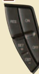
To operate, the speed control must be ON and the vehicle speed must be greater than 30 mph (48 km/h). To set a speed, press SET +. To set a higher speed, press SET + again. To set a lower speed, press SET -. Pressing RES will return to a previously set speed. To turn the speed control off, press the OFF button, or depress the brake pedal to disengage.
