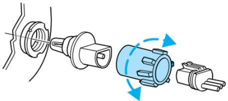
4. Remove the old bulb from the lamp assembly by gently pulling it straight back out of the lamp assembly.
