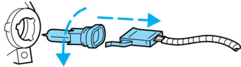
3. Connect the electrical connector to the new foglamp bulb.
