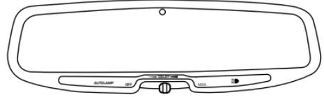
The mirror will automatically return to the normal position whenever the vehicle is placed in R (Reverse) (when the mirror is in the ON position). This helps to ensure a bright clear view in the mirror when backing up.
