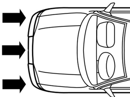
Front air bags are designed to inflate in frontal and near-frontal collisions, not rollover, side-impact, or rear-impacts unless the collision causes sufficient longitudinal deceleration.
