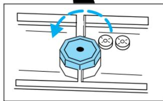
3. Fluid level should be at bottom of the opening.
