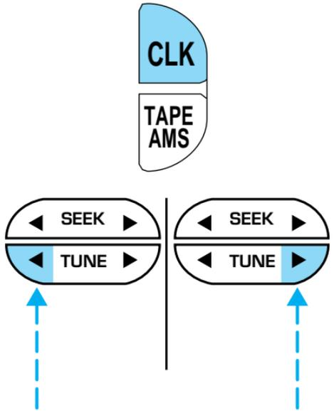
The CLK control will allow you to switch between media display mode (radio station, stereo information, etc.) and clock display mode (time).
