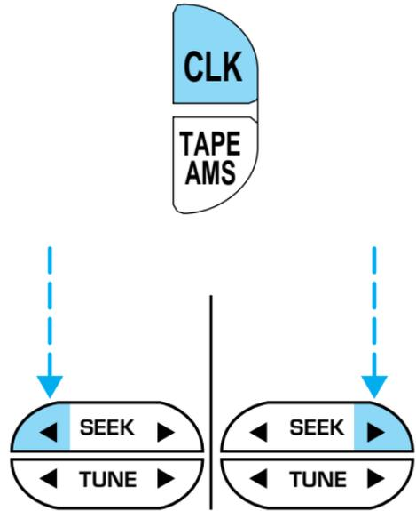
To set the minute, press and hold the CLK control and press the TUNE control:
