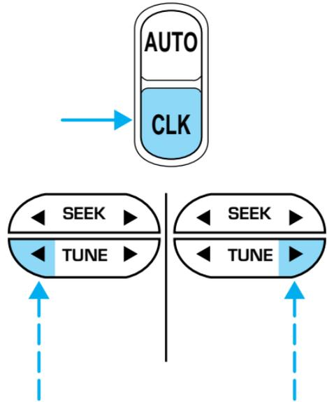
The CLK button will allow you to switch between media display mode (radio station, stereo information, etc.) and clock display mode (time). When in clock mode, the media information will display for 10 seconds, when the radio is turned on, and then revert to clock information. Anytime that the media is changed, (new radio station, etc.), the media information will again display for 10 seconds before reverting back to the clock. In media mode, the media information will always be displayed.
