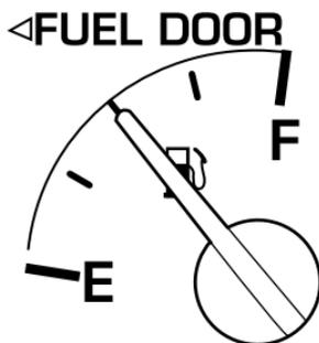
The FUEL DOOR icon and arrow indicates which side of the vehicle the fuel filler door is located.
