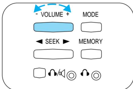
From the rear seat controls, volume control can be set no higher than the current radio setting unless the speakers are turned off. Refer to *Turning speakers on and off*.
