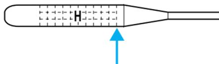
**An overfill condition of transmission fluid may cause shift and/or engagement concerns and/or possible damage.**
