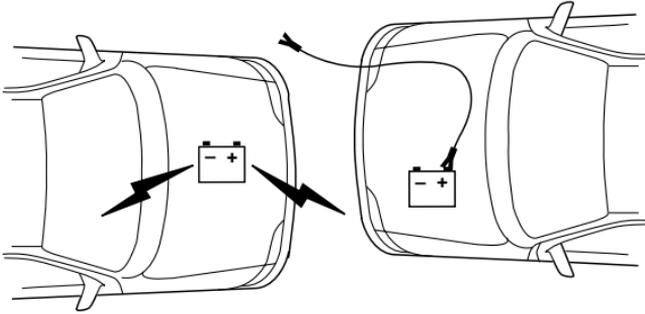
2. Connect the other end of the positive (+) cable to the positive (+) terminal of the assisting battery.
