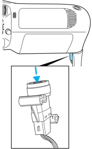
Use the following procedure to reset the fuel pump shut-off switch.
