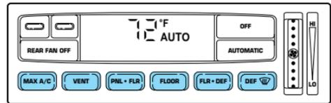
The air conditioning compressor will operate in all modes except FLOOR and VENT. It will also operate only when required when AUTOMATIC has been selected. However, the air conditioning will only function if the outside temperature is about 6°C (43°F) or higher.
