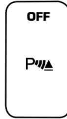
The OFF indicator remains illuminated when the system is disabled. The system defaults to ON every time the reverse gear is selected. Press the control to disable or enable the system.
