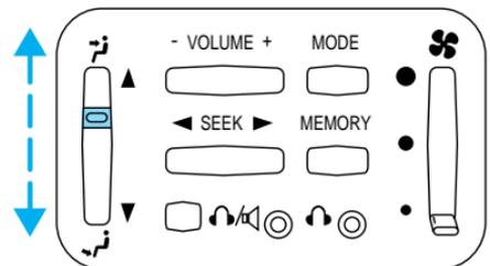
The instrument panel climate controls must be on in order for the rear console climate controls to work.
