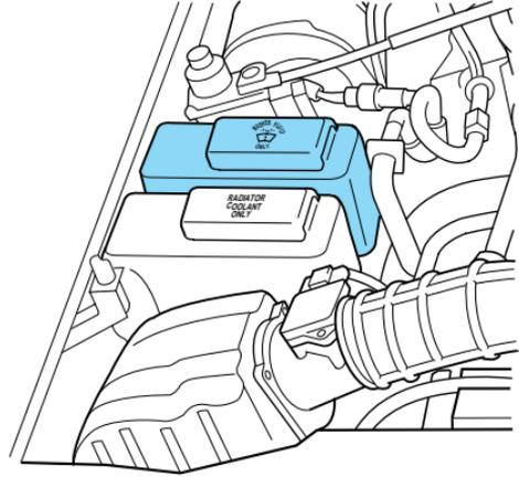
Only use a washer fluid that meets Ford specifications. Refer to *Lubricant specifications* in the *Capacities and specifications* chapter. State or local regulations on volatile organic compounds may restrict the use of methanol, a common windshield washer antifreeze additive. Washer fluids containing non-methanol antifreeze agents should be used only if they provide cold weather protection without damaging the vehicle's paint finish, wiper blades or washer system.
