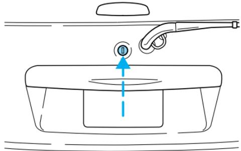
To lock the liftgate and the liftgate window, use the key or the power door locks, depress the key lock cylinder or press the door lock switch on the left side of the cargo area.
