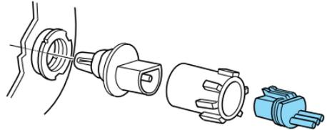
3. Remove the bulb retaining ring by rotating it counterclockwise (when viewed from the rear) to free it from the bulb socket, and slide the ring off the plastic base. Keep the ring to retain the new bulb.
