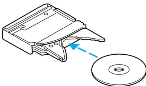
Ensure that the disc holder is evenly inserted and at the same level as the magazine (A). The unit will not operate if the disc holder is not inserted at the same level (B).
