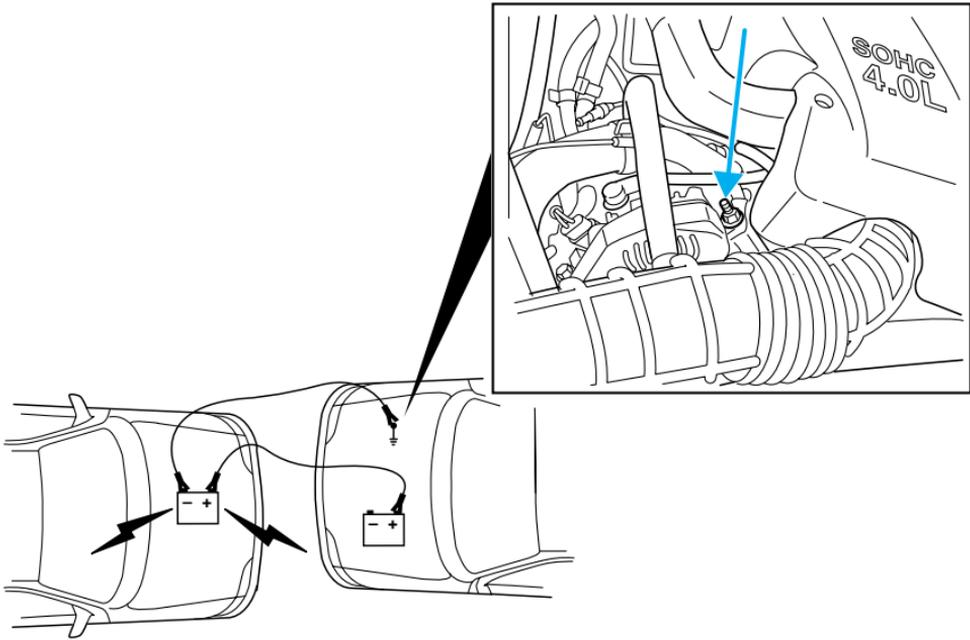
5. Ensure that the cables are clear of fan blades, belts, moving parts of both engines, or any fuel delivery system parts.
