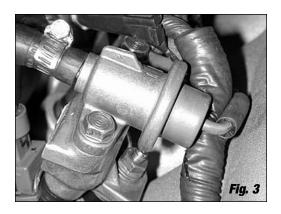
9. Install fuel and vacuum connection along with all needed sensor wires as originally equipped.
