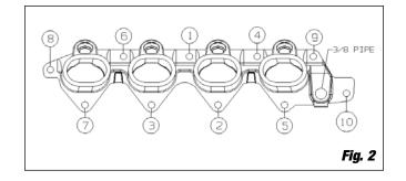
7. Install fuel injectors, stock fuel rail spacers and fuel rail. Each injector should be able to rotate freely after the fuel rail holdown bolts are fully tightened.
