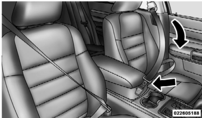
Inserting Latch Plate into Buckle
