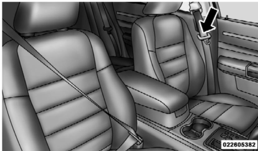
**Pulling Out the Lap/Shoulder Belt Latch Plate**
