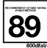
The 5.7L engine is designed to meet all emissions regulations and provide satisfactory fuel economy and performance when using high quality unleaded gasoline having an octane range of 87 to 89. The manufacturer recommends the use of 89 octane for optimum performance. The routine use of premium gasoline is not recommended. The use of premium gasoline will provide no benefit over high quality regular and mid-grade gasolines, and in some circumstances may result in poorer performance.
