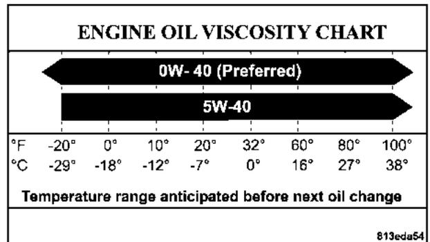
The engine oil filler cap also shows the recommended engine oil viscosity for your engine. For information on engine oil filler cap location, refer to the “Engine Compartment” illustration in this section.
