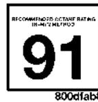
The 6.1L engine is designed to meet all emissions regulations and provide excellent fuel economy and performance when using high-quality premium unleaded gasoline with an octane rating of 91 or higher.
