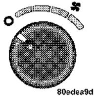
Use this control to regulate the amount of air forced through the system in any mode you select. Turn the control clockwise to increase fan speed. Turn the control to the O — Off position to shut off the fan and to prevent any outside air from entering the vehicle. This also turns off the A/C compressor.
