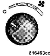
The rotary knob on the left of the control panel is the blower control. Turn the knob clockwise to one of the four positions to obtain the blower speed you desire. To turn the blower off, turn the knob to the far left position.
