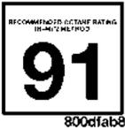
Your vehicle is designed to meet all emission regulations and provide excellent fuel economy when using high quality premium unleaded gasoline having an octane rating of 91 or higher.
