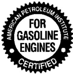
This symbol means that the oil has been certified by the American Petroleum Institute (API). We only recommend synthetic API Certified engine oils, such as Mobil 1®, that meet the requirements of Material Standard MS-10725. Use Mopar or an equivalent oil meeting the specification MS-
