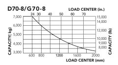
Note: Capacities shown are for trucks equipped with 2-stage view mast up through 197in. (5000mm) maximum fork height, 66.9in. (1700mm) carriage, 48in. (1220mm) forks.
