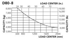
Note: Capacities shown are for trucks equipped with 2-stage view mast up through 197in. (5000mm) maximum fork height, 66.9in. (1700mm) carriage, 48in. (1220mm) forks.
