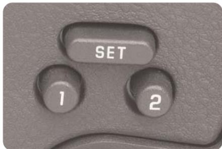
Your vehicle may be equipped with a two-driver memory function that is used to recall memory settings for the driver's seating positions for two drivers. The Driver Information Center (DIC) can also be programmed to personalize additional functions. See the DIC section of this guide for more details.
