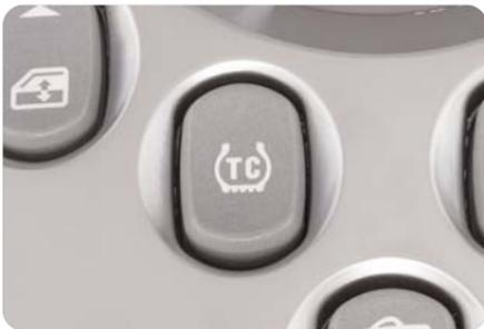
When off, the Traction Control System's "OFF" telltale light will illuminate and remain on. Turn the system back on at any time by pressing the button again. The system will default to ON when the ignition is cycled.
