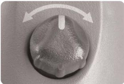
**Power Heated/Automatic Dimming Heated (if equipped):** The power mirror control is located on the driver's door. Turn the knob toward the mirror you wish to adjust, move the knob in the direction you want the mirror to go, and return the knob to the center position. Both mirrors are heated when the rear window defogger is activated, to remove mist and fog.
