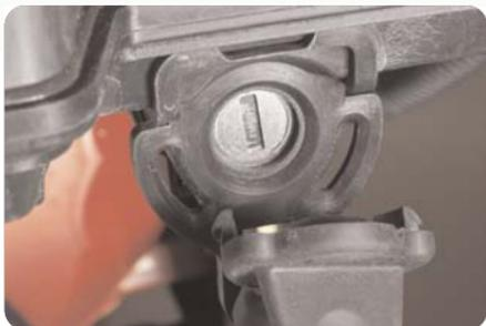
Insert the convertible top release tool (from the glove box) or your ignition key and turn it to activate the emergency release. To remove the cargo cover, see your Owner Manual for full details.
