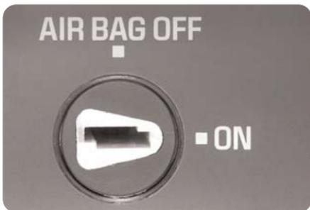
A key-activated switch in the glove box turns off the right-front passenger air
