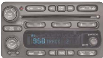
**PWR (Power):** Press this button to turn the system on or off.
