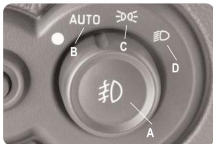
The Fog Lamps button is located in the center of the exterior lamps control ("A" above). Press it to activate or deactivate fog lamps.
