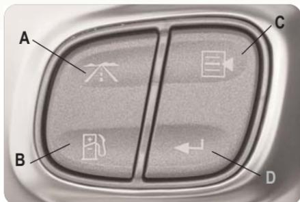
**Trip Information:** Press the Trip Information button (see “A” above) to display the odometer, two trip odometers and the trip timer. To reset the trip odometers or the timer to zero, press and hold the SELECT button (see “D” above) while the desired function is displayed. Use the SELECT button to start and stop the trip timer.
