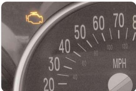
**If the Malfunction Indicator Light is Flashing:** When it is safe to do so, stop the vehicle and turn the engine off. Wait 10 seconds and restart the engine. If the light stays on steadily, see the steps below. If the light continues to flash, follow the previous steps and see your dealer for service as soon as possible.
