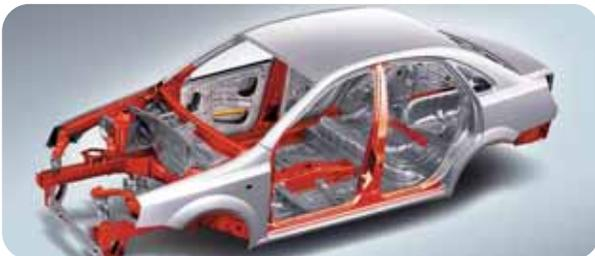
A rigid safety cage made out of high tensile steel protects the passengers and limits the shock of impact.
