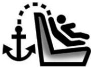
To assist you in locating the top tether anchors, the top tether anchor symbol is located on the cover or near the anchor.
