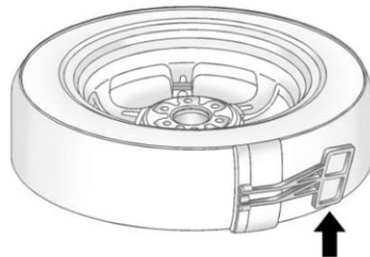
9. Remove the plastic spare tire heat shield by pulling the rubber latch. Store the plastic spare tire heat shield. See “Storing a Flat or Spare Tire and Tools” later in this section for more information.
