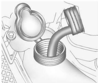
6. Fill the coolant recovery tank to the FULL COLD mark.
