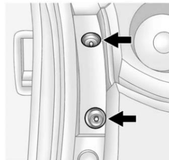
4. Remove the two nuts holding the taillamp assembly in place.
