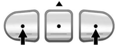
1. From inside the vehicle, press and hold down the two outside buttons at the same time, releasing only when the Universal Home Remote indicator light begins to flash, after 20 seconds. This step will erase the factory settings or all previously programmed buttons.
