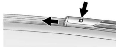
2. Press the button in the middle of the wiper arm connector and pull the wiper blade away from the arm connector.
