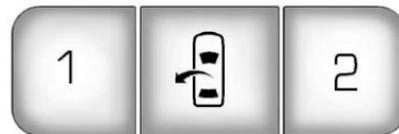
On vehicles with the memory package, the controls on the driver door are used to program and recall memory settings for the driver seat and outside mirrors.
