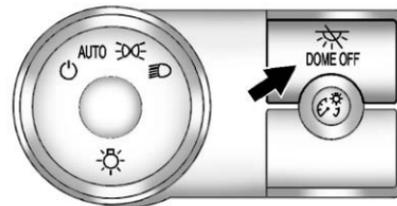
The dome lamp override button is next to the exterior lamps control.
