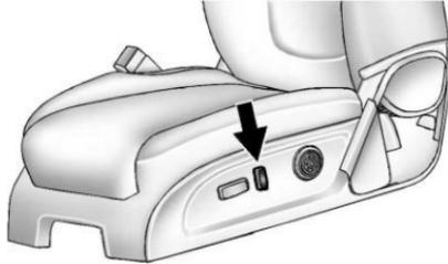
On vehicles with seats that have power reclining seatbacks, the controls used to operate them are on the outboard side of the seats.
