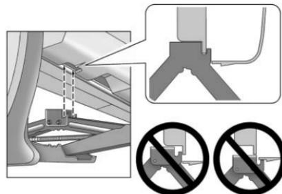
The triangle is located near each wheel on the vehicle's exterior.
