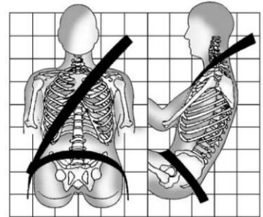
Sit up straight and always keep your feet on the floor in front of you. The lap part of the belt should be worn low and snug on the hips, just touching the thighs. In a crash, this applies force to the strong pelvic bones and you would be less likely to slide under the lap belt. If you slid under it, the belt would apply force on your abdomen. This could cause serious or even fatal injuries.
