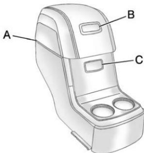
For vehicles with a second row center console, press the buttons (B) or (C) to access storage areas.
