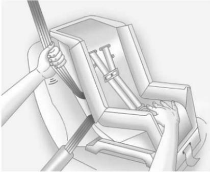
5. To tighten the belt, push down on the child restraint, pull the shoulder portion of the belt to tighten the lap portion of the belt,
