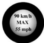
16. If the flat tire was able to inflate to the recommended inflation pressure, remove the maximum speed label from the sealant canister (E) and place it in a highly visible location. The label is a reminder not to exceed 90 km/h (55 mph) until the damaged tire is repaired or replaced.
