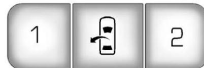
On vehicles with the memory feature, the controls on the driver door are used to program and recall memory settings for the driver seat and outside mirrors.
