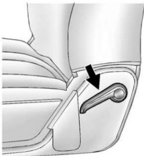
On vehicles with seats that have manual reclining seatbacks, the lever used to operate them is located on the outboard side of the seat.
