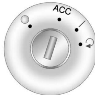
The ignition switch has four different positions.
