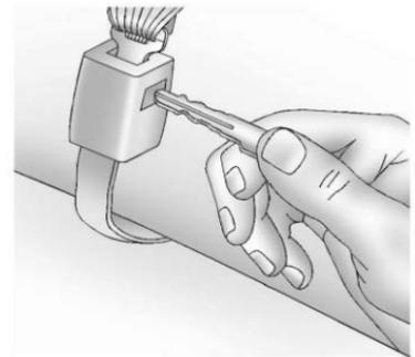
2. Disconnect the rear safety belt mini-latch, using a key in the slot on the mini-buckle, let the belt retract into the headliner. Stow the mini-latch in the holder located in the headliner.
