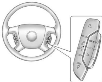
△ / ▽ : Press to change favorite radio stations, select tracks on a CD/DVD, or to navigate tracks or folders on an iPod® or USB device.
