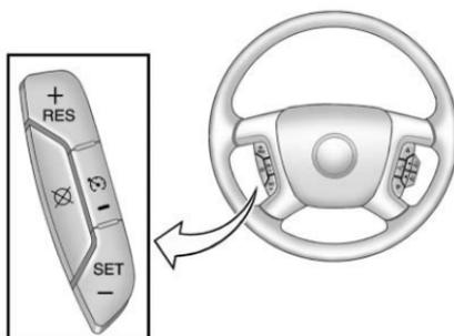
The cruise control buttons are located on left side of the steering wheel.
