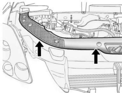
1. Detach fasteners and lift off the panel that covers the radiator cap.
