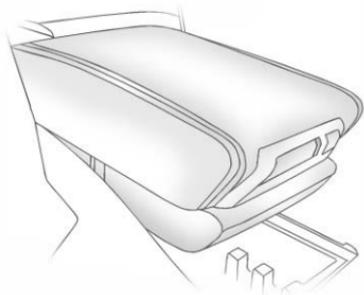
Pull up on the lever, located on the front of the center console armrest, to slide it forward and backward. To open the armrest storage area, press the button located on the front of the armrest. There is additional storage under the armrest. Move the armrest all the way to the rear position, slide the cover back and remove the tray.
