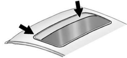
Do not keep the sunroof open for long periods of time while the vehicle is not in use. Dirt and debris may collect on the sunroof seal or in the tracks that could cause an issue with sunroof operation, noise or plug the water drainage system. Periodically open the sunroof and remove any obstacles or loose debris. Wipe the sunroof seal and roof sealing area using a clean cloth, mild soap, and water. Do not remove grease from sunroof.
