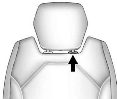
1. Pull the head restraint up to raise it. To lower the head restraint, press the release button, located on the head restraint post on the top of the seatback, while you push the head restraint down.
