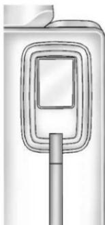
3. Pull up on the release lever located on the back of the seat.
