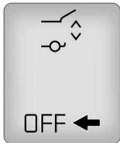
To change the liftgate to manual operation, press the switch on the center console to the OFF position. A message displays, POWER LIFTGATE OFF, to indicate that the liftgate is manual operation. See *Driver Information Center (DIC) (With DIC Buttons)* on page 5-24 or *Driver Information Center (DIC) (Without DIC Buttons)* on page 5-29 for more information.
