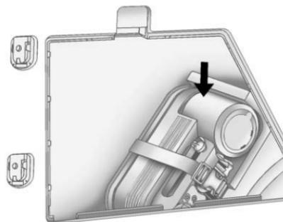
1. Press down on the latch tab and pull the cover off to access the storage compartment.
