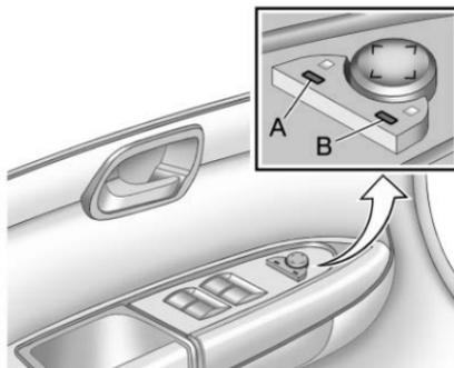
Controls for the outside power mirrors are located on the driver door.
