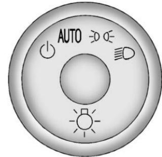
The exterior lamps control is located on the instrument panel to the left of the steering wheel.
