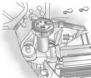
8. Start the engine and let it run until the upper radiator hose feels warm. Any time during this procedure, watch out for the engine cooling fan(s).
