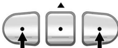
1. Press and hold down the two outside buttons until the indicator light begins to flash, after 20 seconds.
