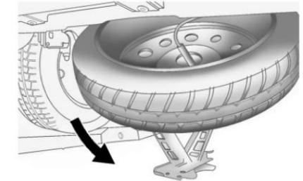
5. Turn the lug wrench clockwise to raise the jack until it lifts the secondary latch spring.
