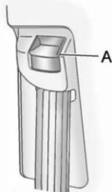
To move it down, push down on the button (A) and move the height adjuster to the desired position. You can move the height adjuster up by pushing up on the shoulder belt guide.
