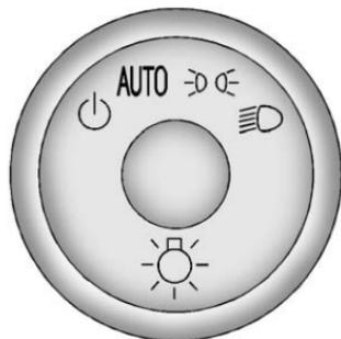
The exterior lamps control is located on the instrument panel, to the left of the steering wheel.
