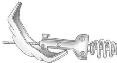
5. Tilt the retainer (F) and slip it through the wheel opening to remove the spare tire (E) from the cable.
