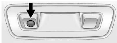
The camera is located in the rear liftgate handle.
