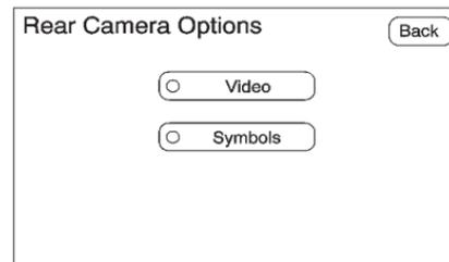
4. Select the Video screen button. When the Video screen button is highlighted the RVC system is on.
