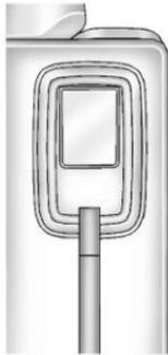
Pull up on the release lever located on the back of the seat and push the seatback forward.
