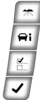
The buttons are the trip/fuel, vehicle information, customization, and set/reset buttons. The button functions are detailed in the following pages.
