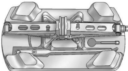
6. Turn the nut holding the jack counterclockwise and remove it. Then remove the jack and wrench.
