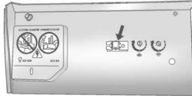
2. In the garage, locate the garage door opener receiver (motor-head unit). Locate the "Learn" or "Smart" button. It can usually be found where the hanging antenna wire is attached to the motor-head unit and may be a colored button. Press this button. After pressing this button, complete the following steps in less than 30 seconds.
