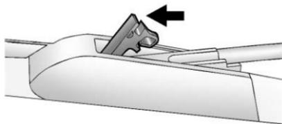
2. While holding the wiper arm, pull the clip up from the blade connecting point, and pull the blade assembly down toward the windshield to remove it from the wiper arm.
