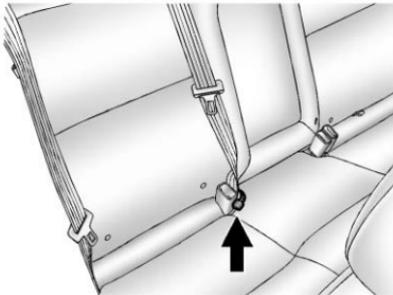
3. Lower the seatback by pulling forward on the tab on the outboard side of the seatback.
