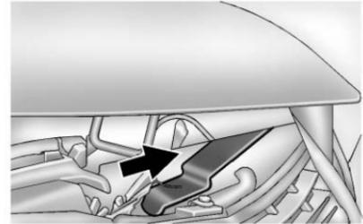
2. Then go to the front of the vehicle and release the secondary hood latch, located near the center of the hood front, by pushing the latch to the right.
