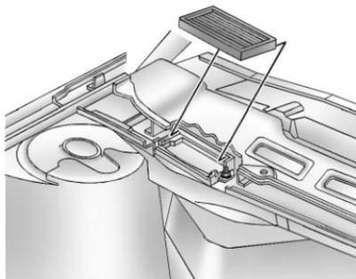
4. Remove the air inlet grille retainers.
