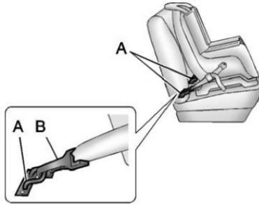
Lower anchors (A) are metal bars built into the vehicle. There are two lower anchors for each LATCH seating position that will accommodate a child restraint with lower attachments (B).
