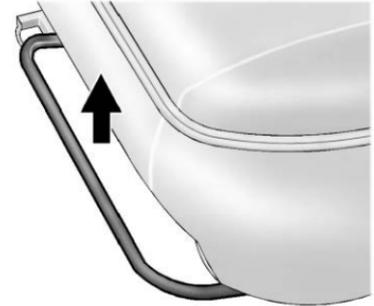
1. Lift the bar under the front edge of the seat cushion to unlock the seat.
