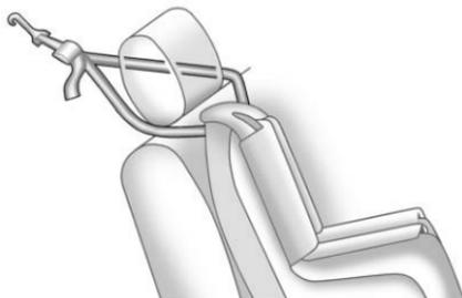
If the position you are using has a fixed headrest and you are using a dual tether, route the tether around the head restraint.
