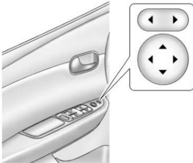
Controls for the outside power mirrors are located on the driver door armrest.
