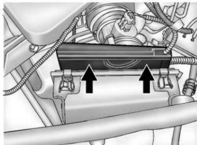
2. Push the filter cover housing toward the engine.
