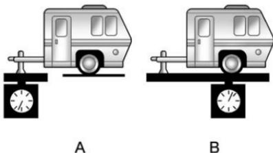
Using a weight-carrying hitch, the trailer tongue (A) should weigh 10 to 15 percent of the total loaded trailer weight (B).
