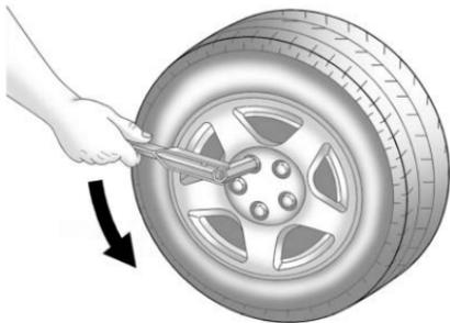
To remove the plastic covers and wheel nut caps, loosen the plastic nut caps with the wheel wrench in a counterclockwise direction.
