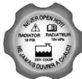
1. Remove the pressure cap when the cooling system, including the pressure cap and upper radiator hose is no longer hot. Turn the pressure cap slowly counterclockwise.
