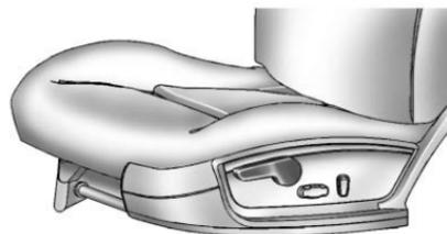
Lift up or push down repeatedly on the lever on the outboard side of the driver seat to increase or decrease lumbar support.
