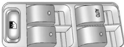
The power window switches are on the driver door armrest. Each passenger door has a switch that controls only that window.
