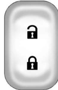
A power door lock switch is located on both front doors next to the door handle.
