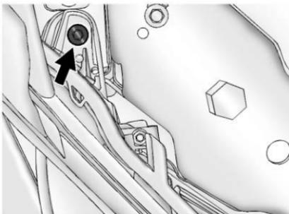
2. Remove the screw from the headlamp assembly.
