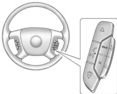
If equipped, these controls are located on the right side of the steering wheel.
