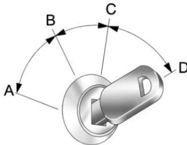
The ignition switch has four different positions.
