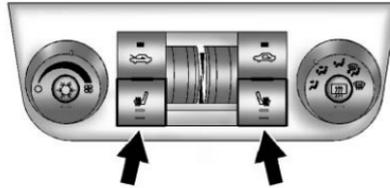
If available, the heated seat buttons are on the climate control panel. The ignition must be on to operate the heated seats.
