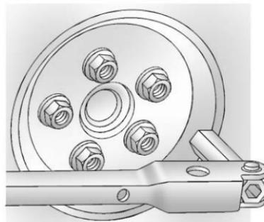
2. Turn the wheel wrench counterclockwise once on each wheel nut to loosen it. Do not remove them yet.
