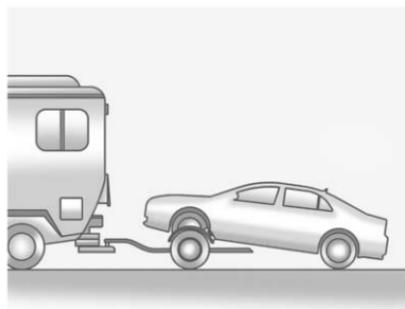
Use the following procedure to dolly tow the vehicle from the front:
