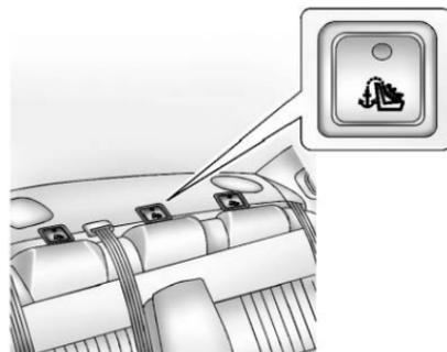
Do not secure a child restraint in a position without a top tether anchor if a national or local law requires that the top tether be attached, or if the instructions that come with the child restraint say that the top tether must be attached.
