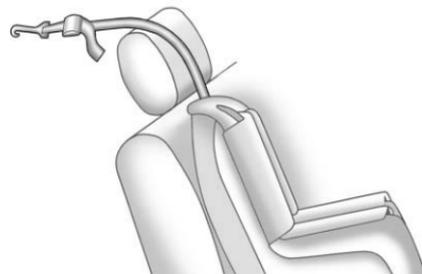
If the position you are using has a fixed headrest and you are using a single tether, route the tether over the head restraint.
