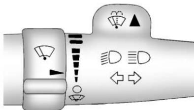
An arrow on the instrument panel cluster will flash in the direction of the turn or lane change.
