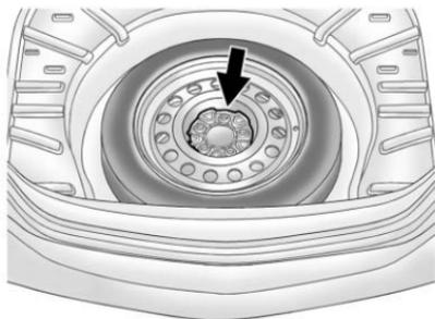
4. Turn the wing nut counterclockwise and remove it.
