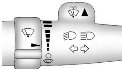
Turn the band with the wiper symbol to control the windshield wipers.
