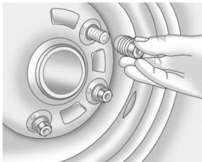
9. Reinstall the wheel nuts with the rounded end of the nuts toward the wheel. Tighten each nut clockwise by hand until the wheel is held against the hub.
