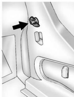
3. Turn the upper wing nut counterclockwise and remove it.
