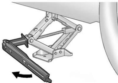
5. Raise the vehicle by turning the jack handle clockwise. Raise the vehicle far enough off the ground to install the compact spare tire.
