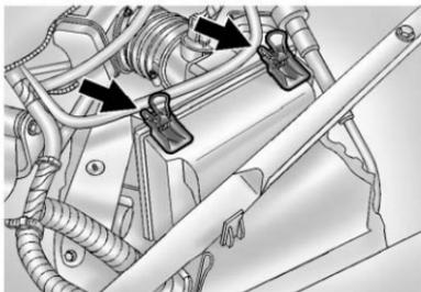
1. Lift the filter cover tabs on top of the engine air cleaner/filter housing.
