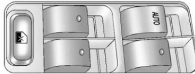
The switches on the driver door armrest are used to control each of the windows. Each passenger door has its own window switch.
