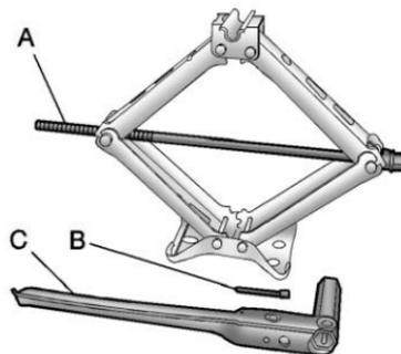
The tools you will need to change a tire include the jack (A), extension and protection guide (B), and wheel wrench (C).
