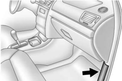
The fuse block is on the passenger side of the vehicle in the carpet molding. Remove the fuse block door to access the fuses.
