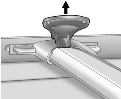
Lift the lever to release and move the crossrail.
