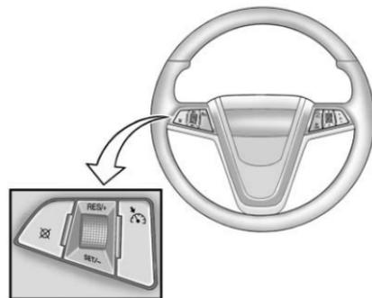
The cruise control buttons are located on the steering wheel.
