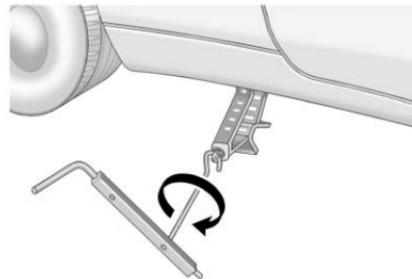
11. Raise the vehicle by turning the jack handle clockwise. Raise the vehicle far enough off the ground so there is enough room for the road tire to clear the ground.
