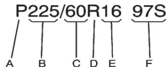
**(A) Passenger (P-Metric) Tire:** The United States version of a metric tire sizing system. The letter P as the first character in the tire size means a passenger vehicle tire engineered to standards set by the U.S. Tire and Rim Association.
