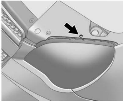
7. Locate the vertical headlamp aiming screws, which are under the hood near each headlamp assembly.
