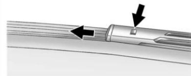
2. Press the square button on the top side, at the end of the wiper arm, and pull the wiper blade out of the end of the wiper arm.
