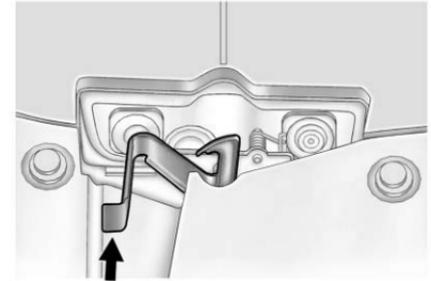
2. Move the secondary hood release lever to the right to release the striker. The lever is near the middle of the hood.
