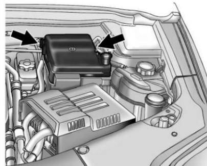
To remove the fuse block cover, squeeze the clips on the cover and lift it straight up.
