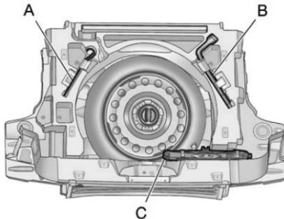
3. Remove the extension (A), wheel wrench (B) and jack (C). Place the tools next to the tire being changed.
