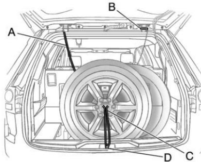
4. Pull the cable (A) through the door striker (D) then the center of the wheel (C).
