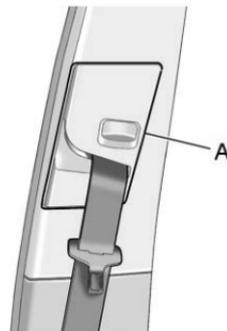
Move the height adjuster up to the desired position by pushing up on the height adjuster.
