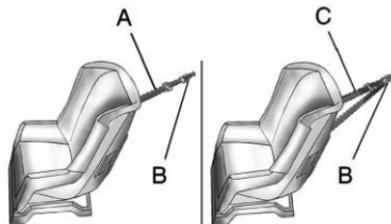
A top tether (A, C) anchors the top of the child restraint to the vehicle. A top tether anchor is built into the vehicle. The top tether attachment (B) on the child restraint connects to the top tether anchor in the vehicle in order to reduce the forward movement and rotation of the child restraint during driving or in a crash.
