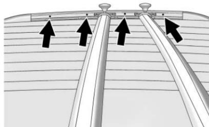
The roof rack crossrails can be locked in four positions along the roof rack side rails.
