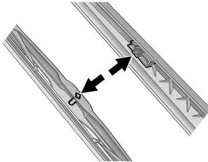
4. Place the wiper blade into the wiper arm aligning the blade attachment rivet with the arm attachment.
