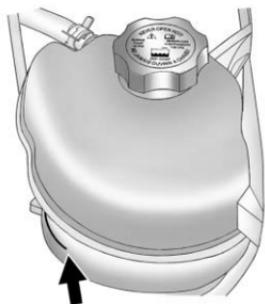
3. Fill the coolant surge tank with the proper mixture to the COLD FILL line.
