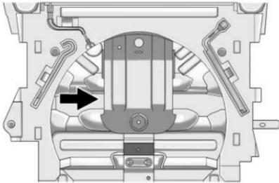
1. Remove the cable package. The cable is stored in a plastic bag under the compact spare tire.
