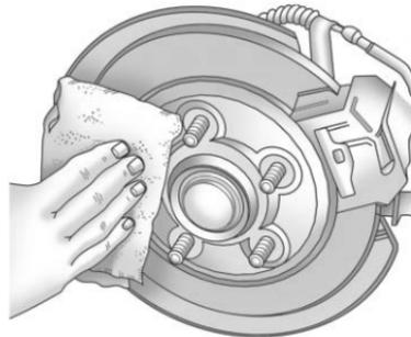
14. Remove any rust or dirt from the wheel bolts, mounting surfaces, and spare wheel.
