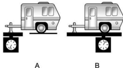
If a weight-carrying hitch or a weight-distributing hitch is being used, the trailer tongue (A) should weigh 10 to 15 percent of the total loaded trailer weight (B).
