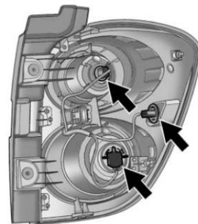
6. Turn the bulb socket counterclockwise and pull it out.
