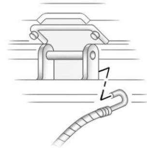
5. Hook the cable onto the outside portion of the liftgate hinges (B).
