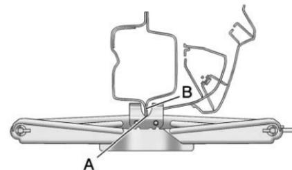
Place the jack notch (A) under the frame rail seam (B).
