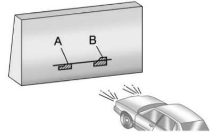
9. Make sure that the light from the headlamp is positioned at the bottom edge of the horizontal tape line. The lamp on the left (A) shows the correct headlamp aim. The lamp on the right (B) shows the incorrect headlamp aim.
