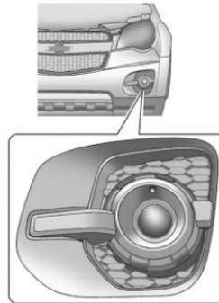
1. Locate the fog lamp assembly under the front fascia.
