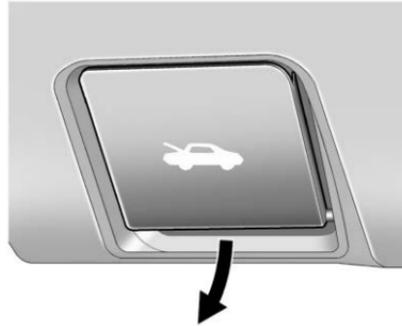
1. Pull the release handle with the symbol on it. It is below the instrument panel, to the left of the steering wheel.
