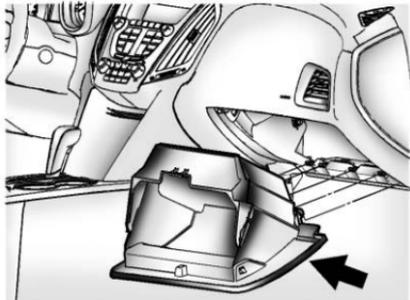
2. Push the stop tab upwards until the stop tab is under the instrument panel assembly and the glove box is released.
