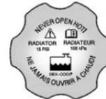
The coolant surge tank pressure cap can be removed when the cooling system, including the surge tank pressure cap and upper radiator hose, is no longer hot.
