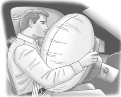
The driver frontal airbag is in the middle of the steering wheel.
