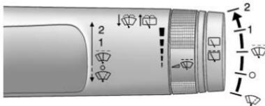
The windshield wiper/washer lever is located on the right side of the steering column.
