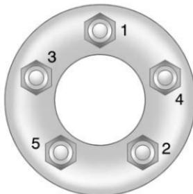
18. Tighten the wheel nuts firmly in a crisscross sequence, as shown.
