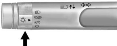
The exterior lamp control is located on the turn signal/lane change lever.
