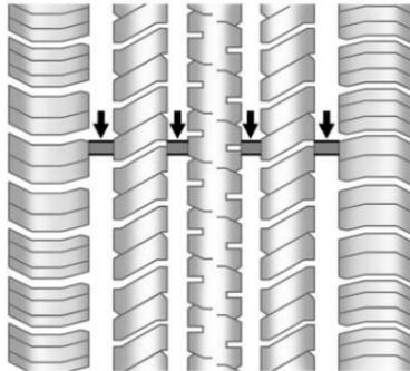
One way to tell when it is time for new tires is to check the treadwear indicators, which appear when the tires have only 1.6 mm (1/16 inch) or less of tread remaining.
