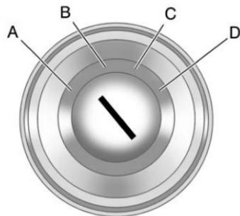
The ignition switch has four different positions.
