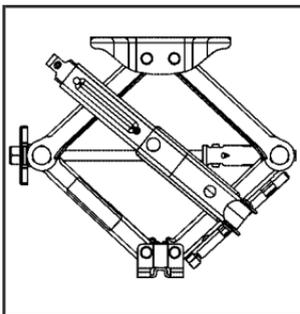
5. Raise the jack to the height shown and lock the wrench onto the jack.
