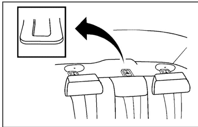
The top tether anchors are located under the covers, behind the rear seat, on the filler panel. Be sure to use an anchor located on the same side of the vehicle as the seating position where the child restraint will be placed.
