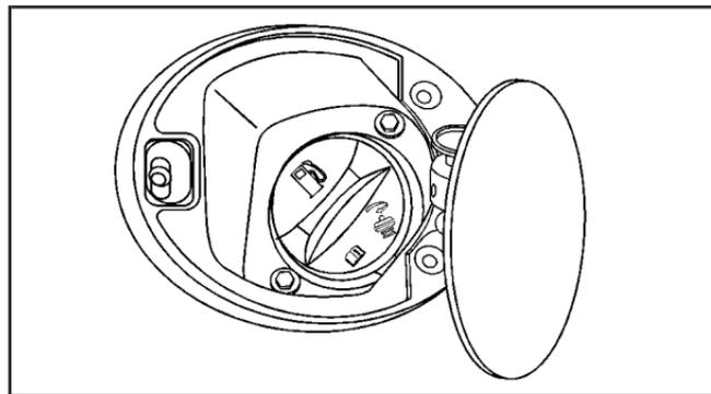
To remove the tethered fuel cap, turn it slowly counterclockwise. If the vehicle has E85 fuel capability, the fuel cap will be yellow and state that E85 or gasoline can be used. See *Fuel E85 (85% Ethanol)* on page 5-8.
