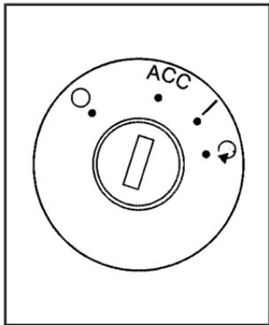
The ignition switch has four different positions.
