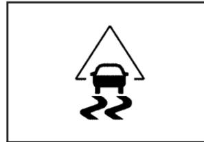
This light will flash on the instrument panel cluster when the ESC system is both on and activated.
