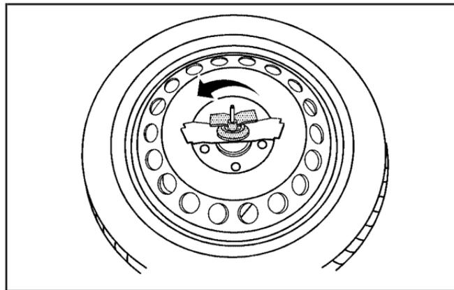
3. Turn the wing nut counterclockwise and remove it. Then remove the compact spare tire. See *Compact Spare Tire* on page 5-89 for more information.
