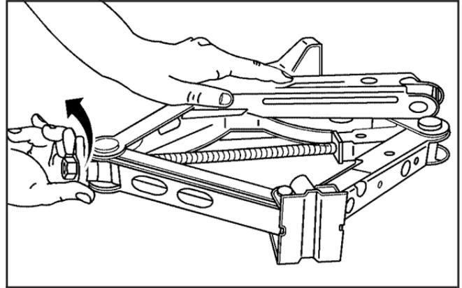
1. Turn the wing nut counterclockwise to loosen wheel wrench.
