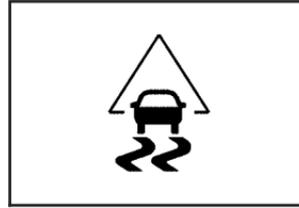
When this light is on solid and either the **SERVICE TRACTION** or **TRACTION OFF** message is displayed, the system will not limit wheel spin.
