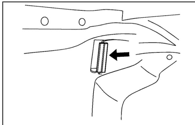
The rear compartment fuse block is located in the trunk of the vehicle. Access the fuse block through the trunk panel on the driver side of the rear cargo area.
