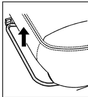
1. Lift the bar to unlock the seat.
