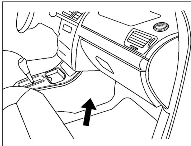
The instrument panel fuse block is located on the instrument panel near the floor on the passenger side of the vehicle.
