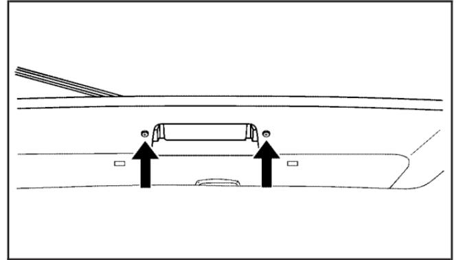
1. Remove the license plate assembly by turning the two screws counterclockwise.
