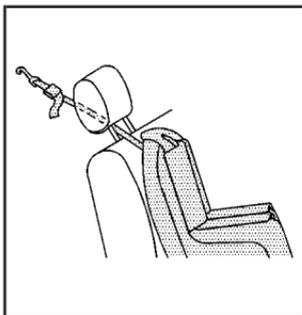
If the position you are using has an adjustable headrest or head restraint and you are using a single tether, route the tether under the headrest or head restraint and in between the headrest or head restraint posts. See *Head Restraints on page 1-2*.
