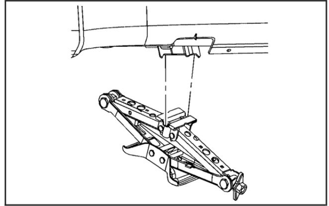
5. Position the lift head at the jack location nearest the flat tire. Make sure all of the jack lift head is touching the jacking flange under the body. Do not place the jack under a body panel.
