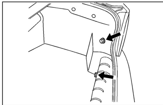
3. Remove the three wing nuts, which hold the taillamp assembly, from inside the vehicle.
