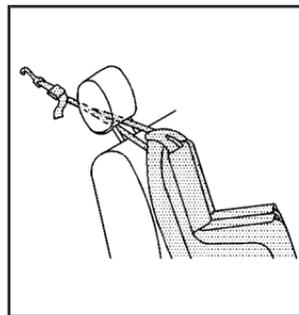
If the position you are using has an adjustable headrest or head restraint and you are using a dual tether route the tether under the headrest or head restraint and in between the headrest or head restraint posts. See *Head Restraints on page 1-2*.
