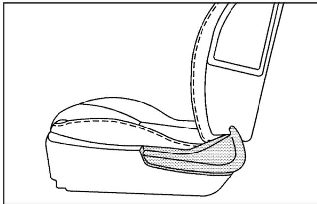
If your vehicle is a coupe or retractable hardtop model, it has a seatback latch as part of the manual recline lever. This feature provides easy access to the rear seats. To operate the seatback latch, pull up on the manual recline lever. The seatback will automatically spring forward. To operate the latch from the rear seat, pull back on the top of the manual recline lever.
