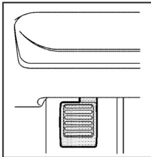
To set the parking brake, push down the parking brake pedal with your left foot. If the ignition is on, the brake system warning light will come on. See *Brake System Warning Light* on page 3-34.
