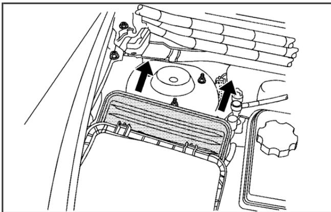
3. Inspect or replace the engine air cleaner/filter.
