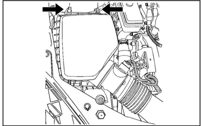
1. Remove the spring clamps that hold the cover on.
