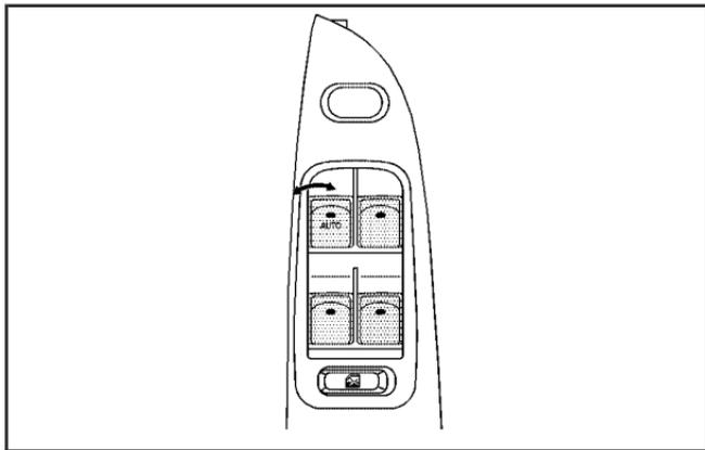
The power window switches are located on the armrest on the driver's door. In addition, there is a switch on each passenger door.
