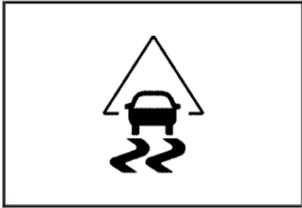
This light will flash when the traction control system is limiting wheel spin.
