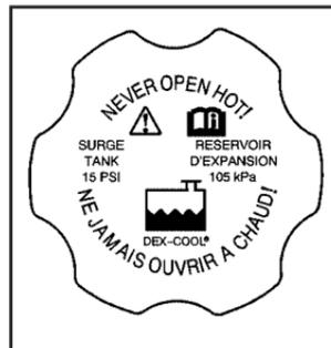
3. Fill the coolant surge tank with the proper mixture, to the FULL COLD mark. Wait about five minutes, then check to see if the level is below the mark. If the level is below the FULL COLD mark, add additional coolant to bring the level up to the mark. Repeat this procedure until the level remains constant at the FULL COLD mark for at least five minutes.
