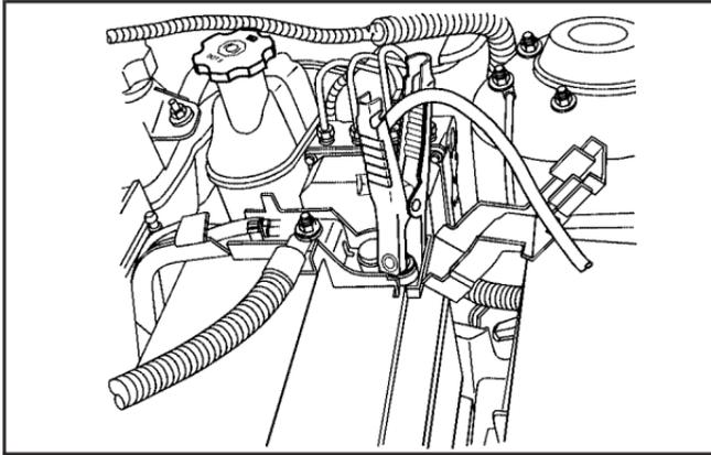
**Notice:** If the jumper cables are connected or removed in the wrong order, electrical shorting may occur and damage the vehicle. The repairs would not be covered by the vehicle warranty. Always connect and remove the jumper cables in the correct order, making sure that the cables do not touch each other or other metal.
