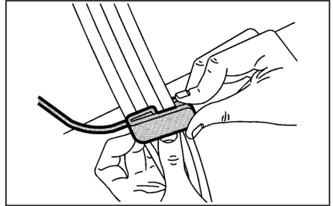
2. Place the guide over the belt and insert the two edges of the belt into the slots of the guide.
