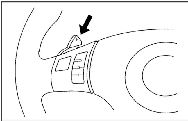
2. Press the + (plus) paddle located on top of the steering wheel controls forward to upshift, or push the backside of the shift paddle rearward to downshift.
