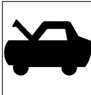
1. Pull the hood release handle with this symbol on it. It is located inside the vehicle to the left of the steering column.
