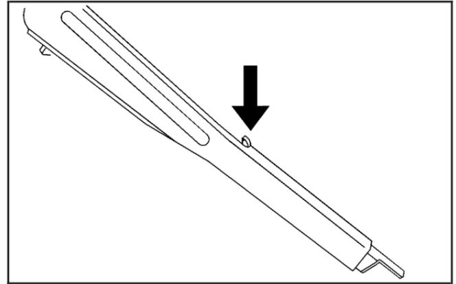
3. Collapse the wrench using the same button used to extend it.
