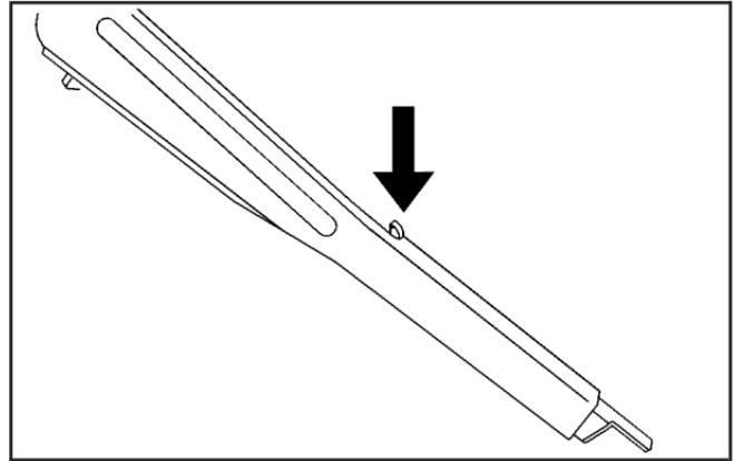
2. Collapse the wrench using the same button used to extend it.
