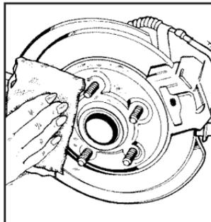
10. Remove any rust or dirt from the wheel bolts, mounting surfaces and spare wheel.
