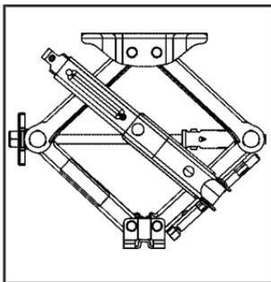
4. Raise the jack to the height shown and lock the wrench onto the jack.
