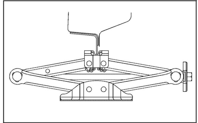
7. Raise the vehicle by turning the wrench clockwise. Raise the vehicle far enough off the ground so there is enough room for the compact spare tire to fit.
