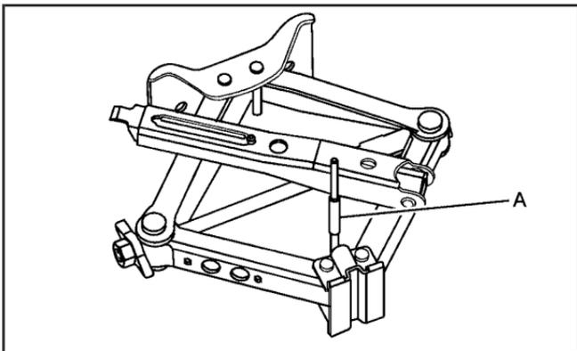
6. Place the jack over the bolt (A) on the floor, making sure it contacts the bolt. Thread the jack retainer nut until it contacts the jack.
