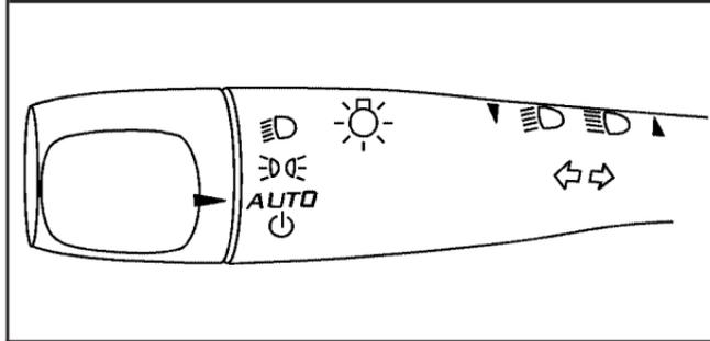
The band on the lever on the outboard side of the steering column operates the exterior lamps.
