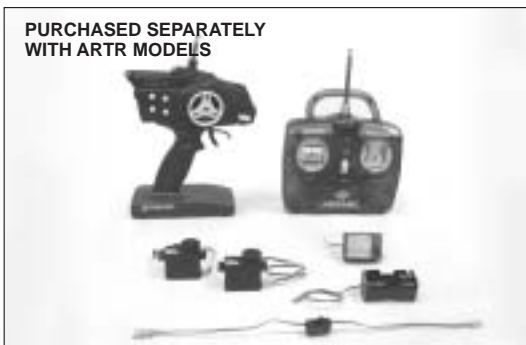
2-Channel, surface radio with 2 high torque servos
