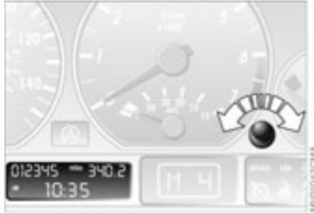
In ignition key position 0: the time is displayed for a few seconds after you press the left button, refer to Odometer on page 71.
