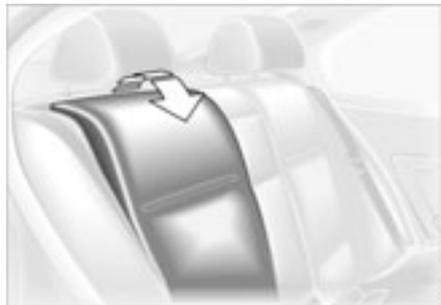
2. The backrest moves forward slightly when released. Reach into the gap and fold it down.
