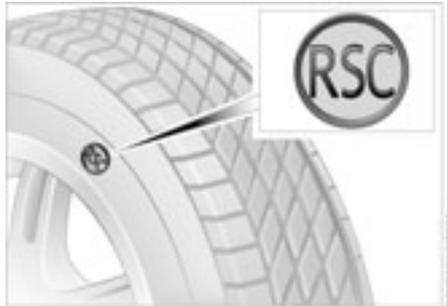
Run Flat tires are labeled on the sidewall with a circular symbol containing the letters RSC. Run Flat tires consist of self-supporting tires and special rims. The tire reinforcement ensures that the tire retains some residual safety in the event of pressure drop and driving remains possible to a restricted degree. The vehicle is equipped with Tire Pressure Monitor (TPM) or Flat Tire Monitor, which indicate a flat tire.
