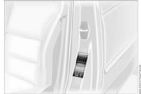
The specified inflation pressures are provided on a sticker attached to the B-pillar and are visible with the driver's door open.
