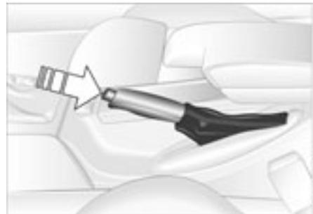
The parking brake is primarily designed to prevent the vehicle from rolling while parked. It operates on the rear wheels.
