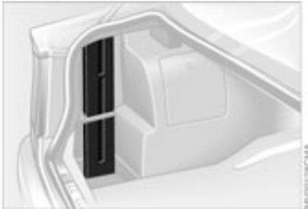
The hazard warning triangle is stored in a storage case on the left side of the luggage compartment.
