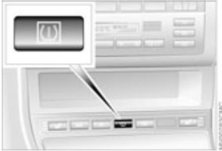
3. Press button as long as you need to until the indicator lamp in the instrument cluster lights up. After a little while, the indicator lamp will go out by itself
