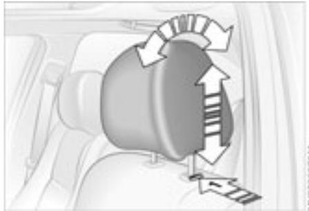
2. Press button – see arrow 1 – and remove the head restraint.
