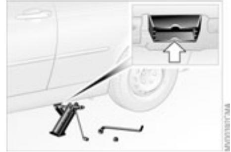
5. Position the jack at the jacking point closest to the flat tire – see arrows – with the jack base vertically below the jacking point and the entire surface of the head of the jack moves into the right-hand corner of the square recess of the jacking point – refer to the detail in the next illustration – when the jack is cranked
