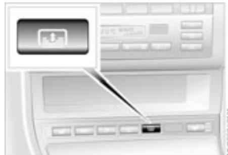
To actuate, press the button briefly with the ignition key in position 1 or higher.
