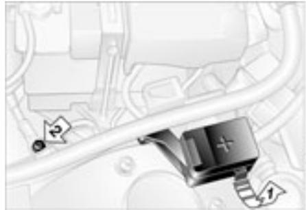
4. The auxiliary jump-starting terminal located in your BMW's engine compartment acts as the positive battery terminal. The cover of this auxiliary terminal is marked with a + sign. Remove by pulling the tab – see arrow 1. Start by connecting the jumper cable from the positive terminal of the discharged battery to the positive terminal of the support battery
