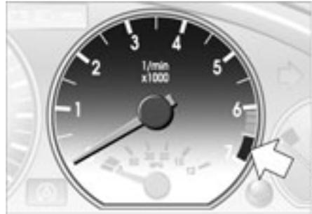
Never allow the engine to operate with the needle in the red overspeed zone of the gauge – see arrow.
