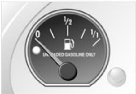
Once the indicator lamp stays on continuously, there are still approx. 2 gallons/8 liters of fuel in the fuel tank. Fuel tank capacity approx. 16.6 gallons/63 liters.
