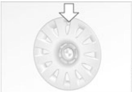
13. Wheels with full wheel covers\*: place the wheel cover with the valve opening – see arrow – over the valve. Use both hands to press the cover securely onto the rim
