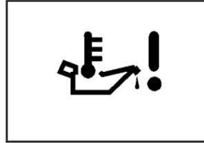
When you see this flashing symbol, the engine oil temperature is high.
