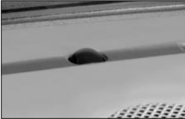
The light sensor for the DRL and AUTO headlamp feature is located on top of the instrument panel. If you cover the sensor, it will read dark, and the exterior lamps or the Headlamps Suggested message will appear on the DIC whenever the ignition is on.
