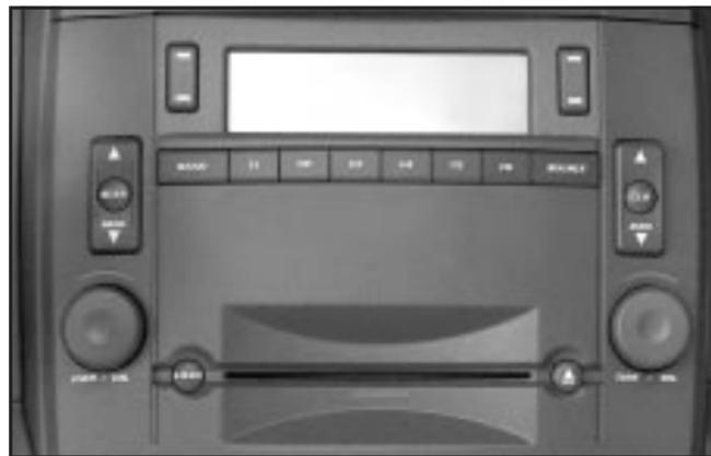
Use the following controls located on the audio system to operate the DIC:
