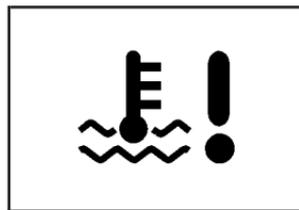
When you see this flashing symbol, the engine coolant temperature is high (257°F (125°C)).
