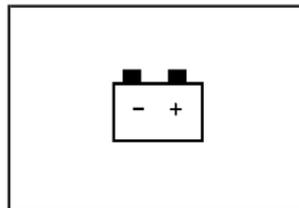
When you turn the key to ON or START, this light will come on briefly to show that the generator and battery charging systems are working properly.
