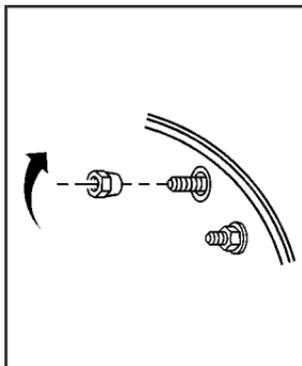
11. Put the wheel nuts back on with the rounded end of the nuts toward the wheel. Tighten each wheel nut by turning it clockwise with your hand until the wheel is held against the hub.
