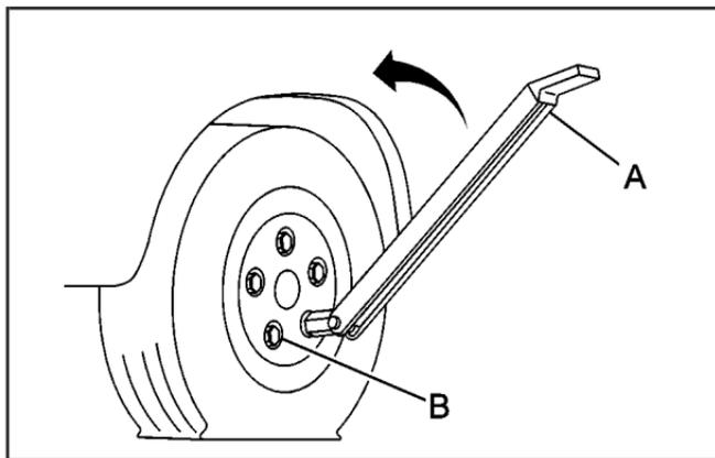
1. Place the wheel wrench (A) securely over the wheel nut (B). Turn the wheel wrench counterclockwise to loosen all the wheel nuts. Don't remove them yet.
