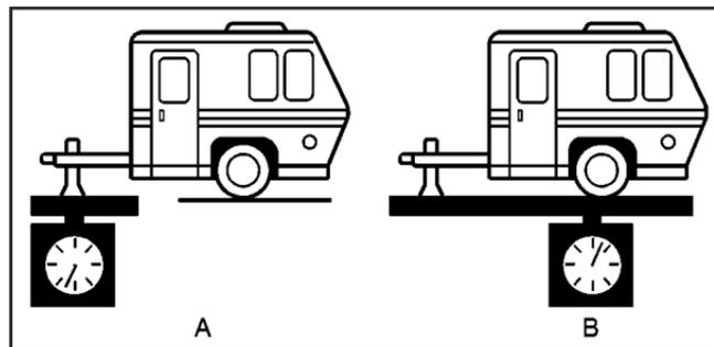
If you're using a weight-carrying hitch or a weight-distributing hitch, the trailer tongue (A) should weigh 10 to 15 percent of the total loaded trailer weight (B).
