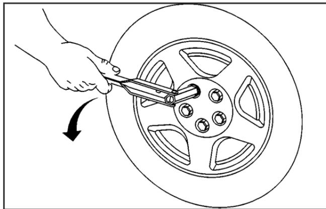
If your vehicle has wheel nut caps, turn the wheel wrench counterclockwise to remove the caps.
