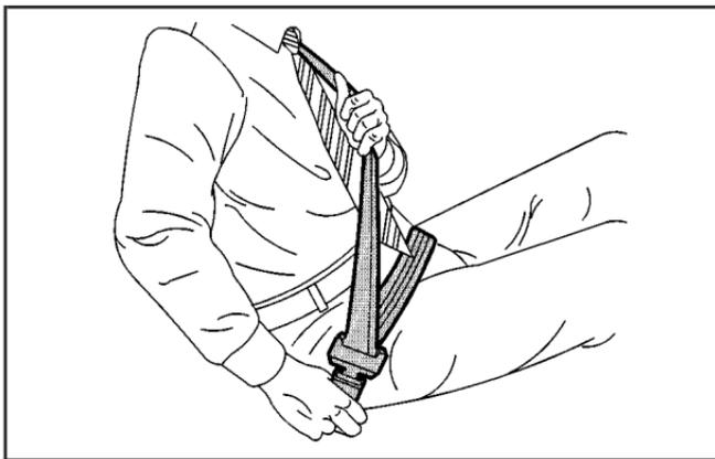
5. To make the lap part tight, pull down on the buckle end of the belt as you pull up on the shoulder belt.
