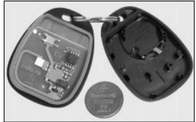
3. Insert the new battery as the instructions under the cover indicate.
