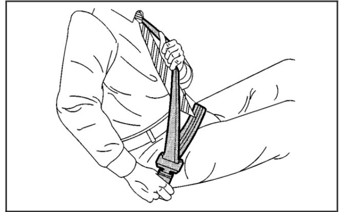
3. To make the lap belt part tight, pull down on the buckle end of the belt as you pull up on the shoulder part.
