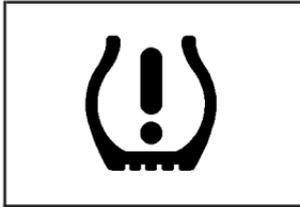
When you see this flashing symbol, one or more of the vehicle's tires is either under or over-inflated.
