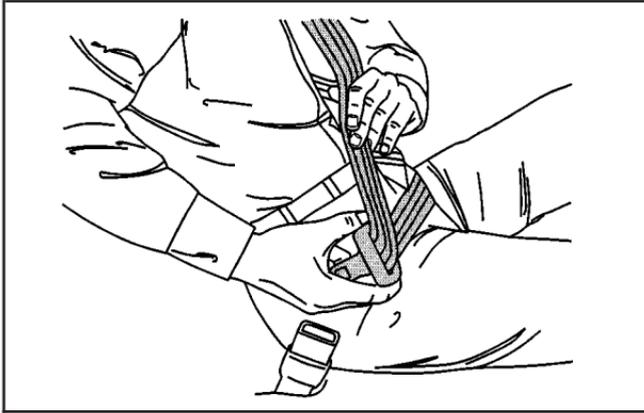
If the belt stops before it reaches the buckle, tilt the latch plate and keep pulling until you can buckle it. Pull up on the latch plate to make sure it is secure. If the belt is not long enough, see *Safety Belt Extender* on page 1-27.
