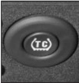
You can turn the system off by pressing the TC (traction control) button located in the glove box.
