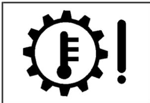
When you see this flashing symbol, the transmission fluid temperature is high (290°F (143°C)).
