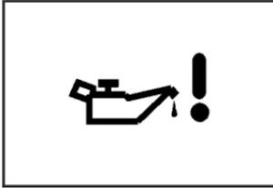
When you see this flashing symbol, the engine oil pressure is low.
