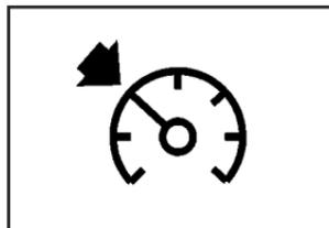
This light on the instrument panel cluster will come on when cruise control is on. It will go out when cruise control is turned off.
