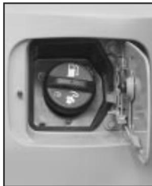
The tethered fuel cap is located behind a hinged fuel door on the passenger's side of the vehicle. To open the fuel door, push inward on the forward edge of the fuel door until the rear edge can be pulled outward.
