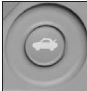
The remote trunk release button is located on the lower portion of the driver's door.
