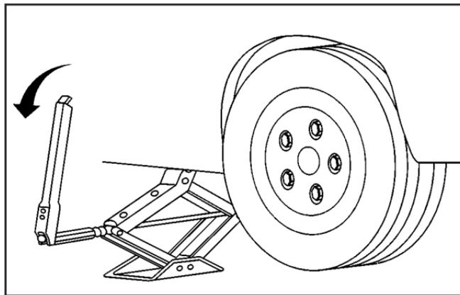
12. Lower the vehicle by turning the wheel wrench counterclockwise. Lower the jack completely.
