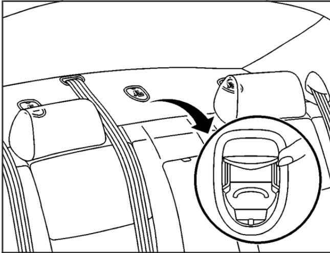
The top strap anchors are located on the filler panel behind the rear seat head restraints. In order to access the anchors, you will have to open the covers.
