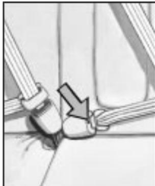
1. Insert a tool with a small tip into the slot as shown to unlatch the seatbelt buckle. Then move the belt to the side so it is not in your way.
