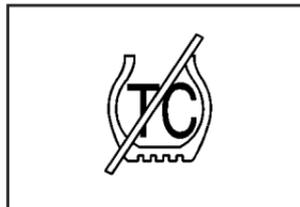
You can turn the system off by pressing the TC (traction control) button located on the steering wheel.
