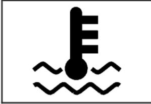
When the coolant temperature is displayed you will see the coolant temperature symbol.
