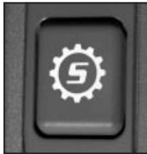
The sport mode button is located on the center console near the transmission shift lever.
