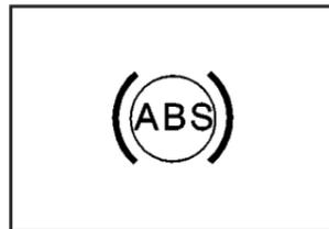
If there is a problem with the anti-lock brake system, this warning light will stay on. See *Anti-Lock Brake System Warning Light* on page 3-43.
