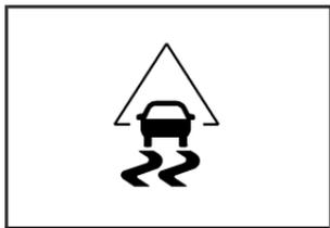
The traction control system warning light should come on briefly when the engine is started.
