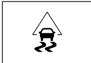
For vehicles that have the StabiliTrak<sup>®</sup> system, this warning light should come on briefly when the engine is started.
