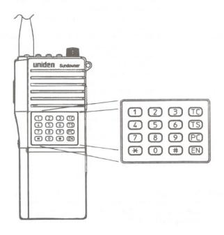
① to ② : NUMERIC Keys; Used to select channels, enter special Receiver/Transmit Codes and other SELCALL Parameters
