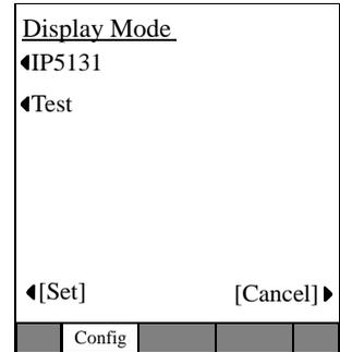
The IP5131 setting allows default operation of the display as it was designed to support 10 LCD keystrips plus 4 lines of call processing/softkey information.
