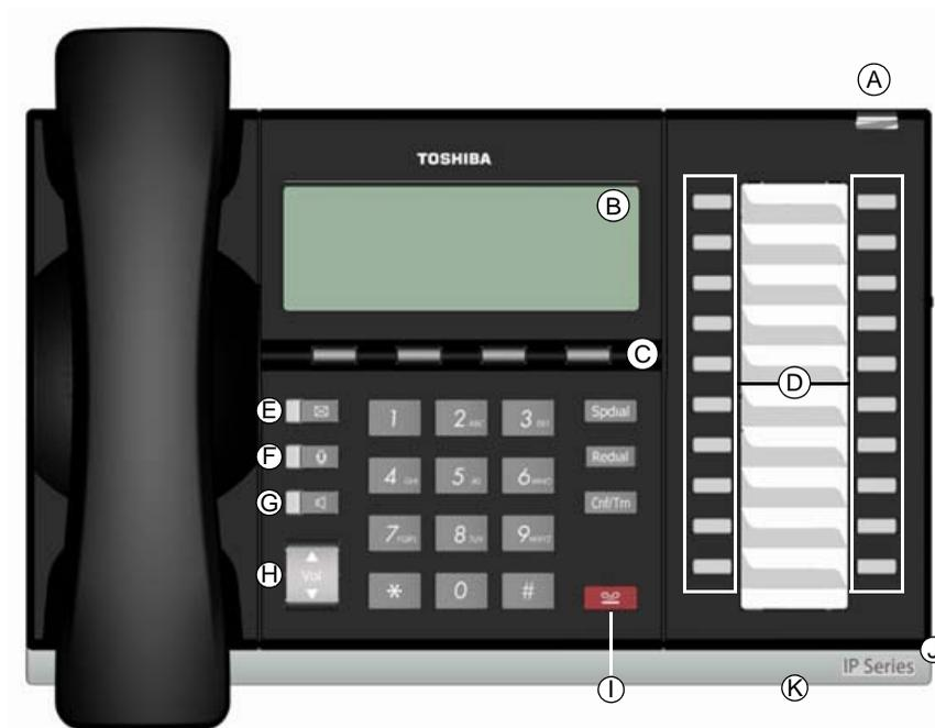
20 Programmable Feature Buttons 4-Line LCD Telephone
