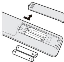
Remove the back cover to reveal the battery compartment and make sure the batteries are inserted the proper way. Suitable battery types for this remote control are AAA, IEC R03 1.5 V.
