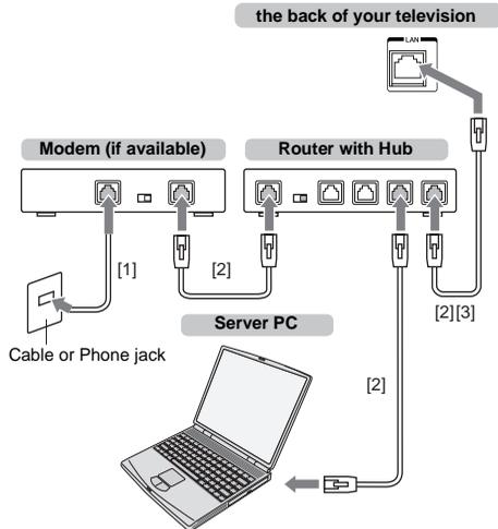
[1] Coaxial or telephone cable (depending on your modem type)
