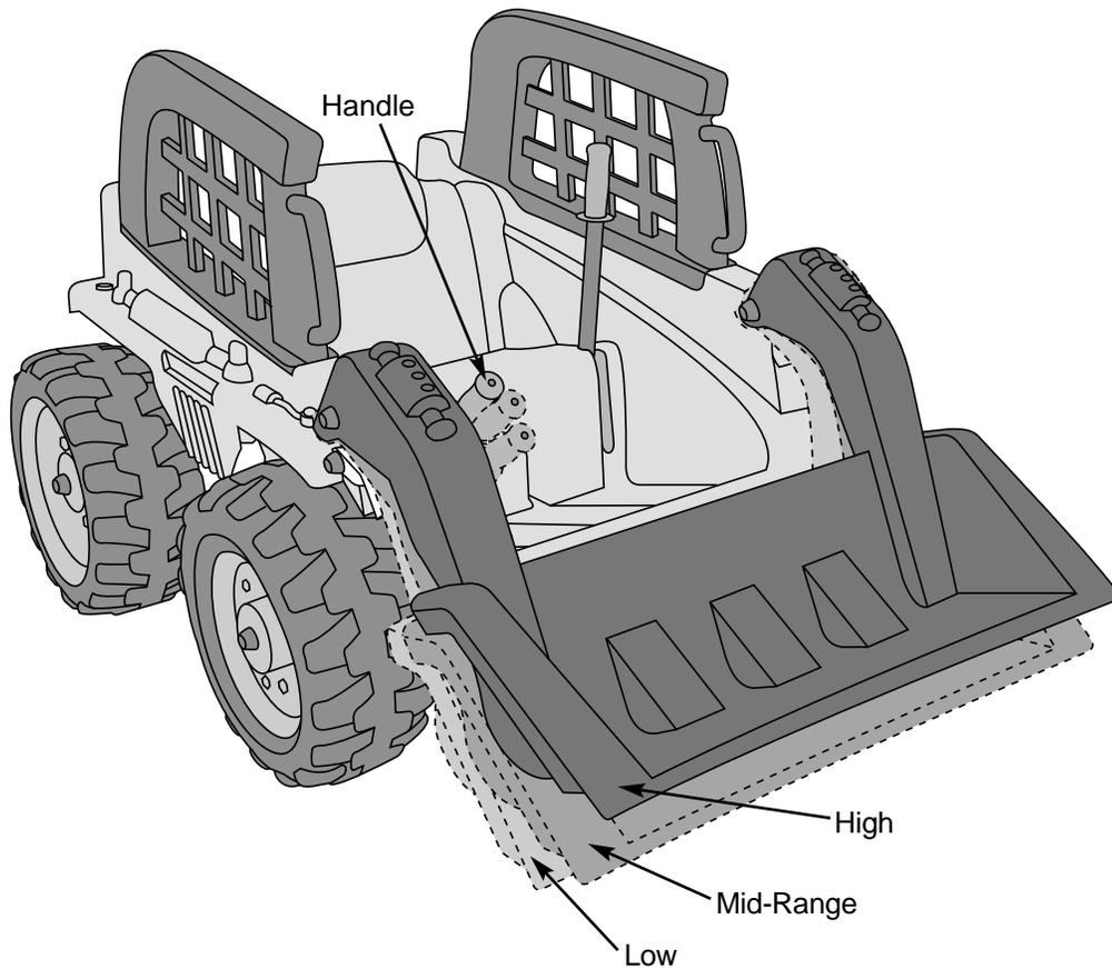
**IMPORTANT!** The bucket is designed to automatically drop to its lowest position with a load that exceeds 10 lbs. **Do not** modify the bucket to defeat this safety feature.
